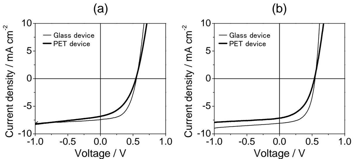
**Figure 4** Photo I-V curves of the inverted polymer solar cells on glass or PET substrate with MEA-ZnO (a) or AA-ZnO layer (b) as electron collection layer. Heat treatment of ZnO film for the glass device was at 250°C and for the PET device at 100°C.
