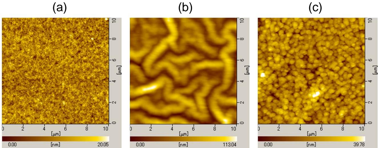
**Figure 3** Surface AFM images of the sol-gel ZnO films on glass or PET substrate prepared by various heat treatments; (a) MEA-ZnO, 250°C, glass, (b) MEA-ZnO, 100°C, PET and (c) AA-ZnO, 100°C, PET.
