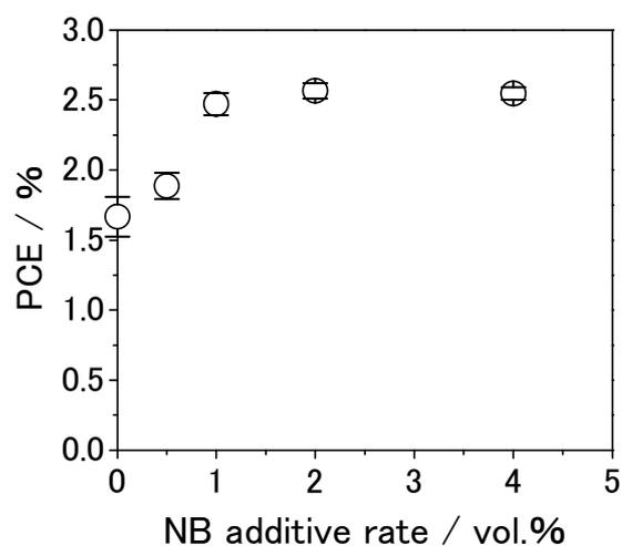
**Figure 5** Plots of PCE of the flexible inverted polymer solar cells containing PCBM:P3HT blend film prepared using CB:NB solvent, against vol. % of NB added.
