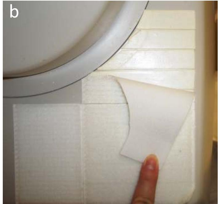
**Fig. 6a-b.** Traces of the exfoliation of hook-and-loop fasteners off powerful double-sided tapes for plastic.
