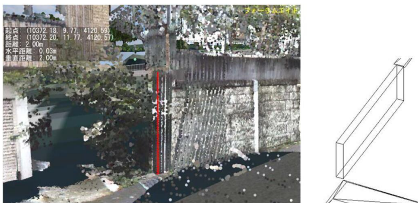
Figure 9. Neighboring fence's height is reflected in the BIM model
