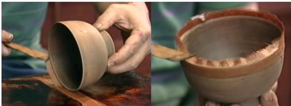
5. Applying lacquer to the base. This step should be repeated 15-20 times to gain the best quality. The application of lacquer to the base consists of the application of *shitaji*, *fuki urushi*, and *uwanuri*.
