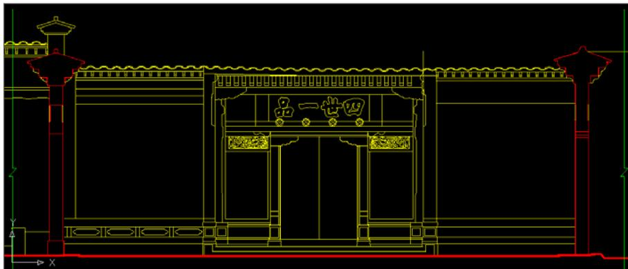
Figure 2-9 The vertical face drawing of the entrance
