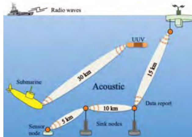
Figure 2.16. Underwater communicating nodes using acoustic links (L. Emokpae, 2013)
