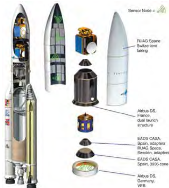
Figure 2.14. Wireless sensor technology placement and deployment plan for Ariane 5's upper stage
