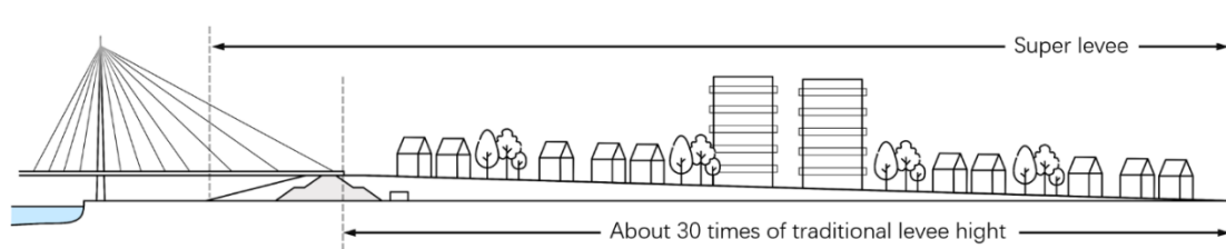
Figure 3.7 Concept of Super Levee
