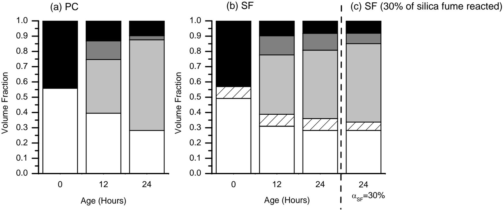
Fig.3 Volume fractions of constituent phases in concretes
