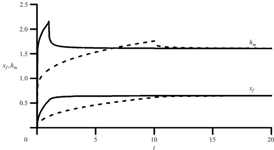
FIGURE 10. Time variation of the maximum height ( $h_m$ ) and the front location ( $x_f$ ). Solid lines :  $Q_0 = 1$ ; broken lines :  $Q_0=0.1$ . The total volume is  $V_0 = 1$ . Discharge is terminated at  $t = T_0 = 1$  and  $10$ , respectively. Note the rapid decrease of  $h_m$  when discharge ends.
