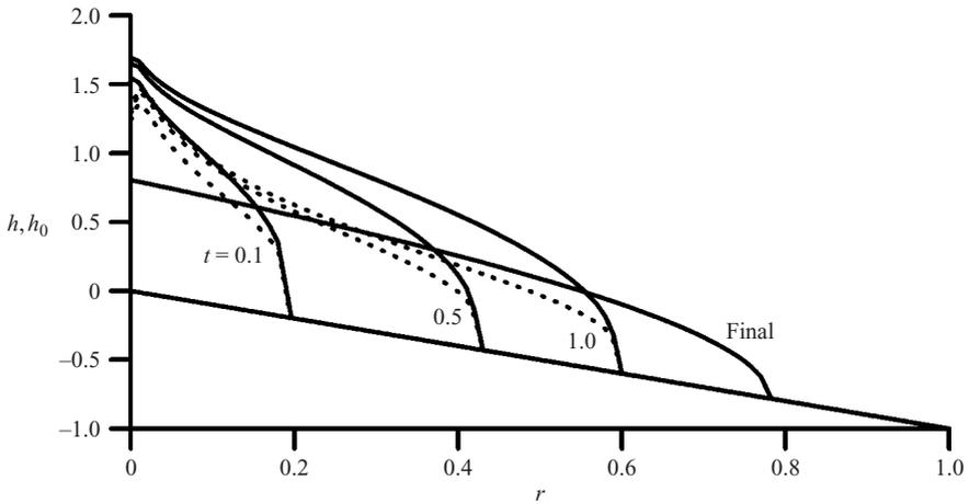
FIGURE 17. Time evolution of the free surface and the yield surface for  $V_0 = 1$  and  $Q_0 = 1$ . The source is at  $x_s = 0, y_s = 0$  (axisymmetric spreading). Solid line: free surface; dashed line: yield surface. The final free surface is at  $t = 20$ . The final yield surface coincides with the solid bottom.
