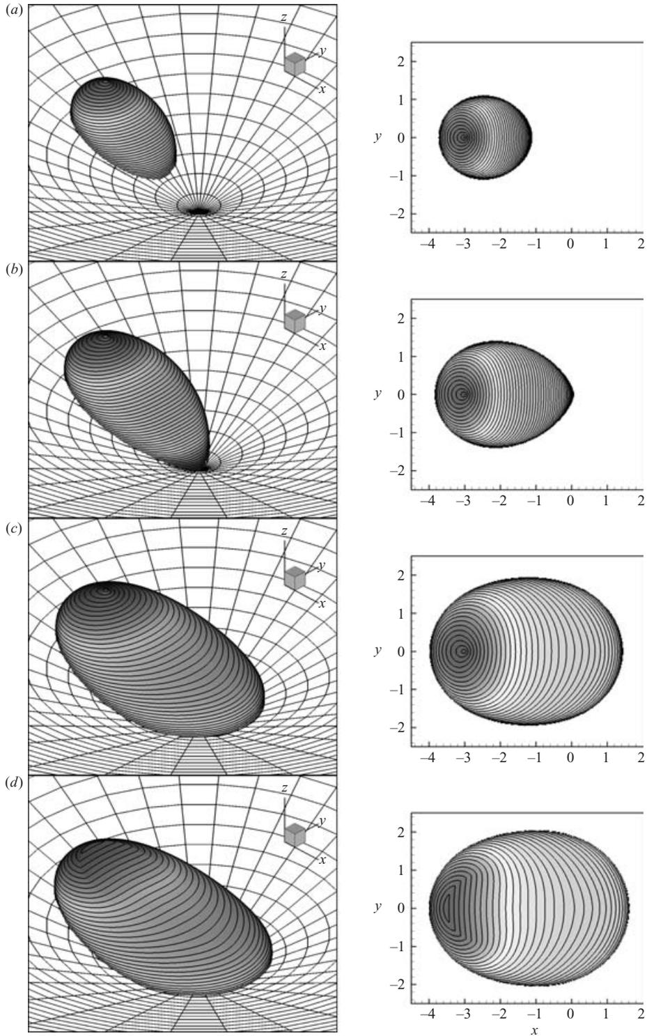
FIGURE 12. Time evolution of mudflow for  $V_0 = 27$  and  $Q_0 = 1$ . (a)  $t = 5$ , (b) 10, (c) 27, (d) 100. The source is at  $x_s = -3$ ,  $y_s = 0$ . Discharge is terminated at  $t = 27$ . In the right-hand column the contour lines of the free surface height are plotted with the interval  $\Delta h = 0.1$ . The highest contour is (a)  $h = 5.0$ , (b)  $h = 5.1$ , (c)  $h = 5.2$ , (d)  $h = 4.8$ , respectively.
