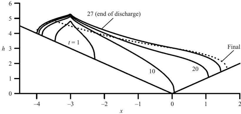
FIGURE 14. Time evolution of the centreline profile for  $V_0 = 27$  and  $Q_0 = 1$ . The mud is discharged from  $t = 0$  to  $t = 27$ . The source is at  $x_s = -3, y_s = 0$ . The final profile is obtained at  $t = 500$ .
