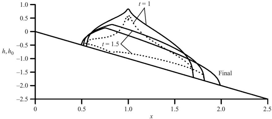
FIGURE 19. Time evolution of the free surface and the yield surface for  $V_0=1$  and  $Q_0=1$ . The source is at  $x_s = 1$ ,  $y_s = 0$ . Solid line: free surface; dashed line: yield surface. The final free surface is at  $t = 20$ . The final yield surface coincides with the solid bottom.
