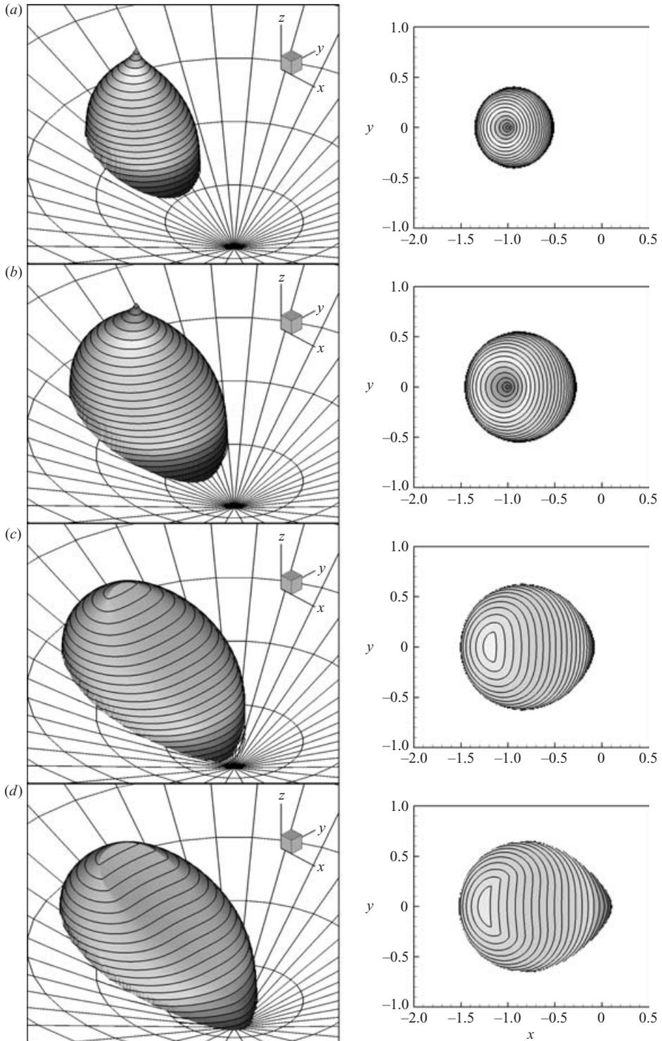
FIGURE 11. Time evolution of mudflow for  $V_0 = 1$  and  $Q_0 = 1$ . (a)  $t = 0.5$ , (b) 1, (c) 2, (d) 20. The source is at  $x_s = -1$ ,  $y_s = 0$ . Discharge is terminated at  $t = 1$ . In the right-hand column the contour lines of the free-surface height are plotted with the interval  $\Delta h = 0.1$ . The highest contour is (a)  $h = 2.7$ , (b)  $h = 2.8$ , (c)  $h = 2.2$ , (d)  $h = 2.1$ , respectively.
