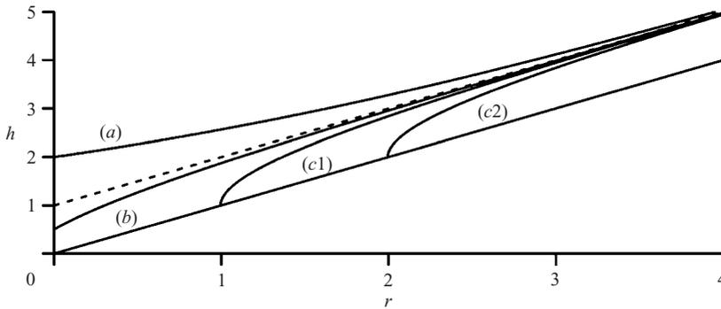
FIGURE 5. Downward threshold in conical basin. (a) sample case for  $h_* > 1$  ( $h_* = 2, r_* = 0$ ), (b) sample case for  $h_* < 1$  and wet bottom ( $h_* = 0.5, r_* = 0$ ). The broken line denotes the case of uniform thickness  $h_* = 1, r_* = 0$ , (c) sample cases for partially dry bottom, (c1):  $R = 1$ , (c2):  $R = 2$ .
