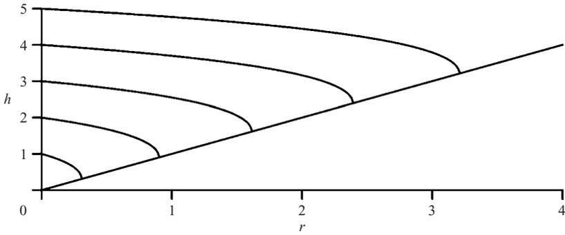
FIGURE 3. Upward thresholds in a conical basin for various maximum depths at the centre. In normalized form, all profiles near the edge are the same.
