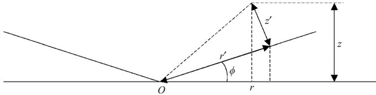
FIGURE 20. Relations between conical coordinates  $(r', \theta', z')$  and cylindrical polar coordinates  $(r, \theta, z)$ . Only the vertical cross-section is shown. The azimuthal angle  $\theta' = \theta$  is taken as in the ordinary polar coordinates.
