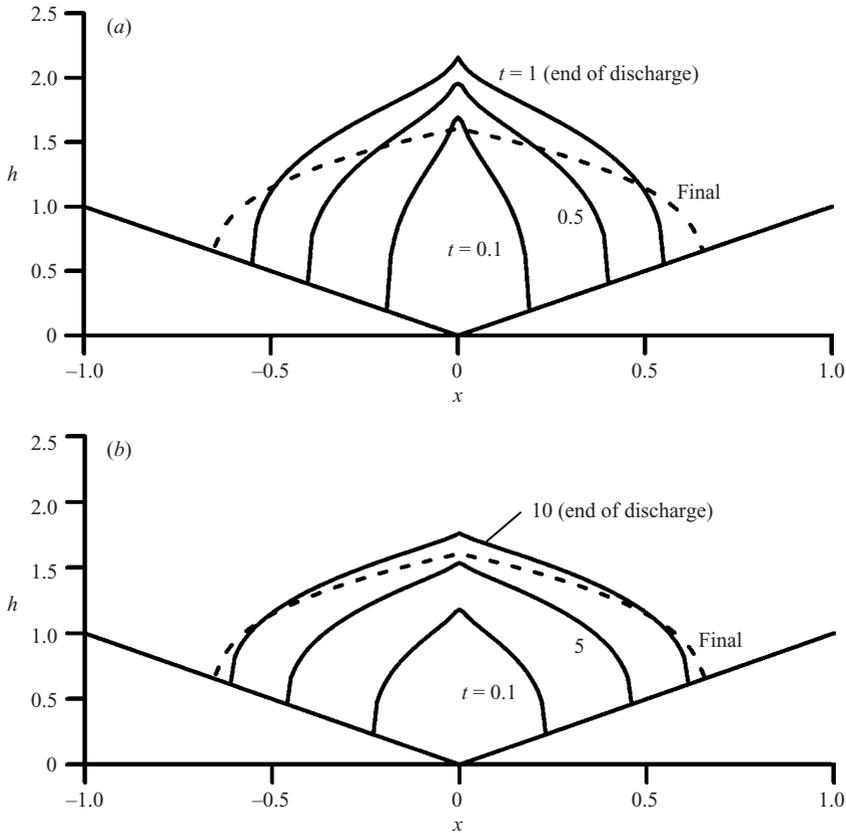
FIGURE 9. Time evolution of the free surface for  $V_0 = 1$ . The source is at  $x_s = 0, y_s = 0$  (axisymmetric spreading). Discharge is terminated at  $t = T_0 = 1$  and 10, respectively. (a)  $Q_0 = V_0/T_0 = 1$ . (b)  $Q_0 = V_0/T_0 = 0.1$ .
