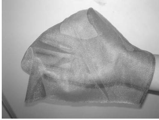
Fig. 3. Electro-magnetic shield cloth.
