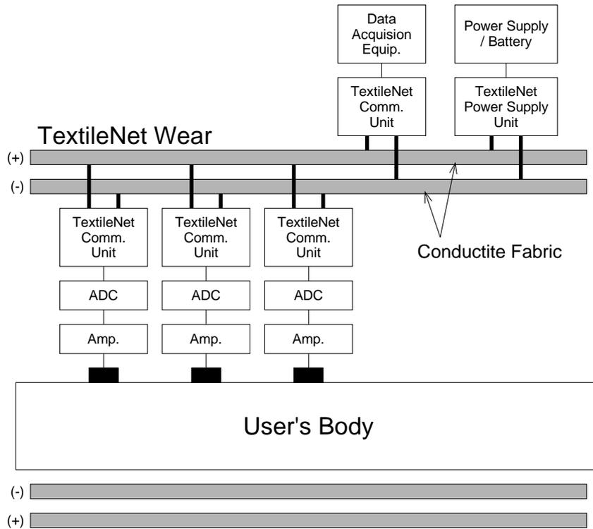
Fig. 16. Configuration of EMG measurement system using TextileNet.
