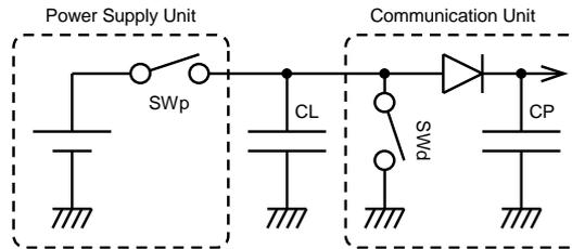
Fig. 4. Circuit architecture of data communication and power supply unit of TextileNet.
