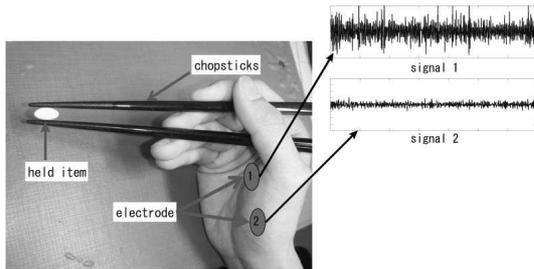
Figure 4: Experimental view (B: hold position (state that maintains the power of the finger))
