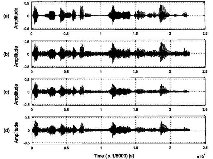
Fig. 8. Waveforms of the simulation result. (a) Clean speech. (b) Noisy speech ( $SNR'_{in} = 5$  dB). (c) Enhanced speech with the LMS algorithm as the NRF ( $SNR'_{out} = 5.95$  dB). (d) Enhanced speech with the LLMS algorithm of  $\alpha_{LLMS} = 0.001$  as the NRF ( $SNR'_{out} = 6.20$  dB).
