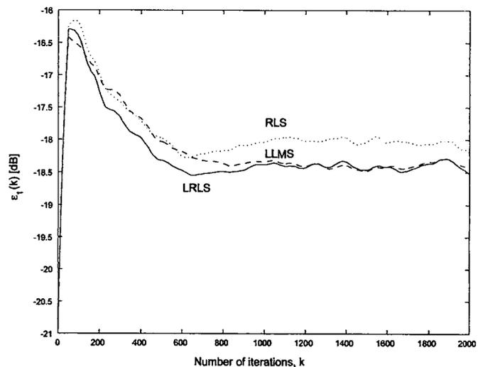
Fig. 4. Comparison of the experimental result  $\epsilon_1(k)$  of the LRLS and the LLMS algorithms with the RLS algorithm of the same initial condition for  $b_1 = 0.4$ .
