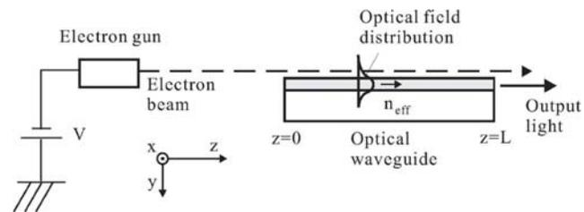
Fig.1 Configuration of the optical emitter
