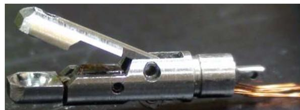
Fig.6. Constructed gripper
