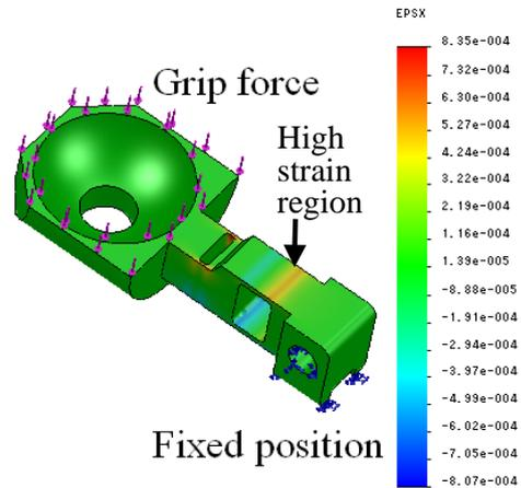
Fig.4. Strain analysis on the detection clip
