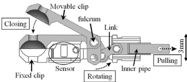
Fig.2. Setup of the gripper
