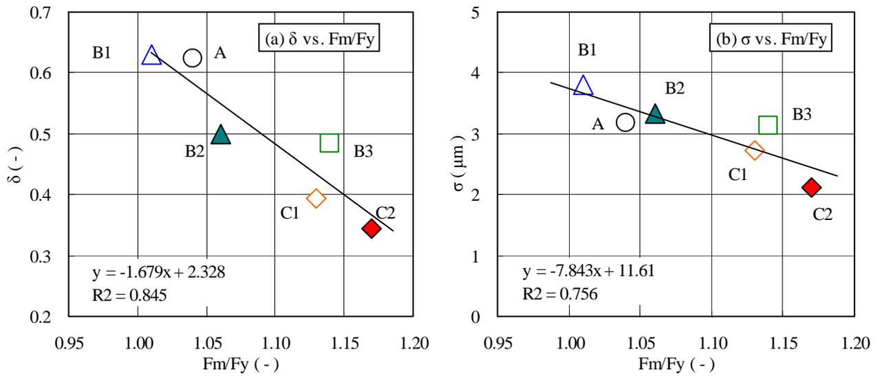
Fig.12 Relationship between Fm/Fy and film thickness uniformity parameter (a) $\delta$ , (b) $\sigma$
