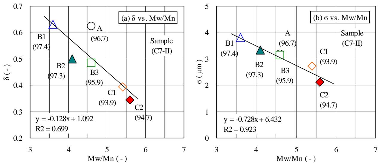
Fig.14 Relationship between Mw/Mn and film thickness uniformity parameter (a) $\delta$ , (b) $\sigma$
