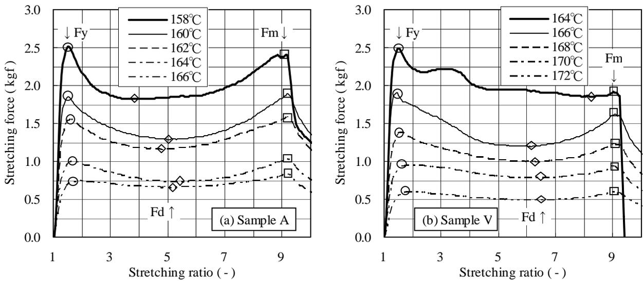
Fig.5 Stress -strain curve of (a) sample A and (b) sample V at several stretching temperatures
