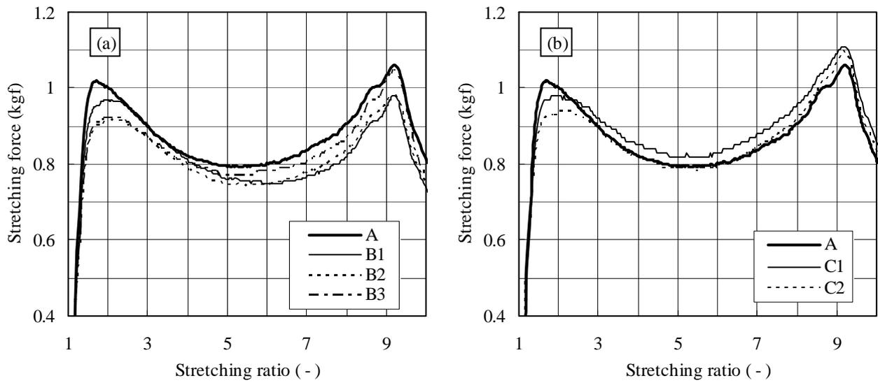
Fig.8 Strain-Stress curve of (a)low crystallinity samples and (b)wide MWD samples
