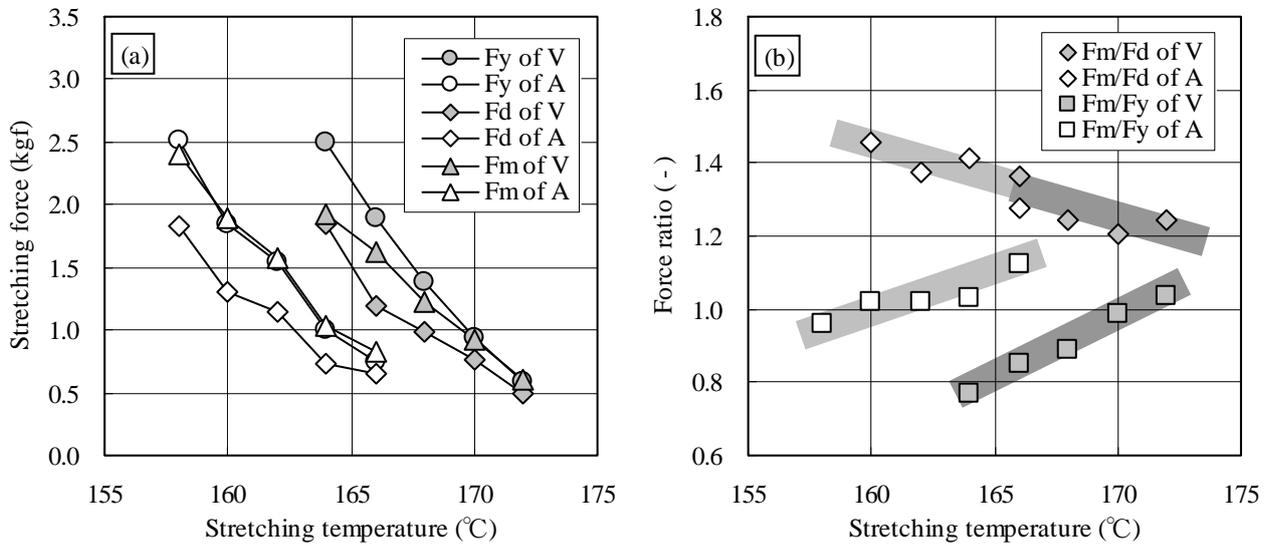
Fig.7 (a) Stretching force and (b) stretching force ratio of sample A and V
