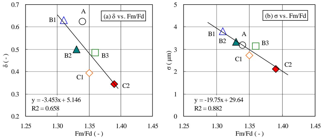
Fig.13 Relationship between Fm/Fd and film thickness uniformity parameter (a) $\delta$ , (b) $\sigma$
