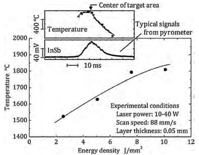
Fig. 5. Variation of temperature with energy density.
