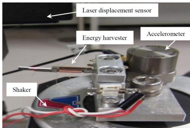
Fig. 9. Measurement setup
