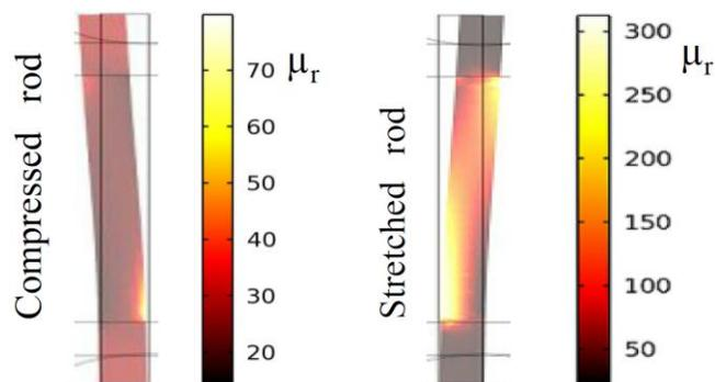
Fig. 7. Spatial variations of relative permeability inside the Galfenol rod.
