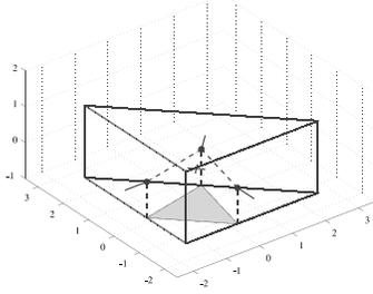
Figure 6: Optimal Grasp Points in Case III
