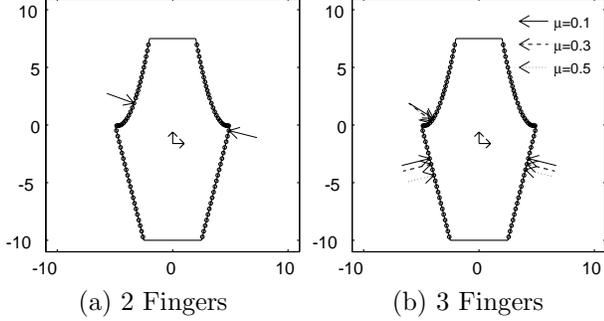
Figure 5: Optimal Grasp Points in Case II
