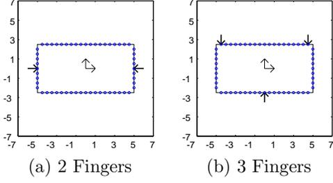
Figure 4: Optimal Grasp Points in Case I
