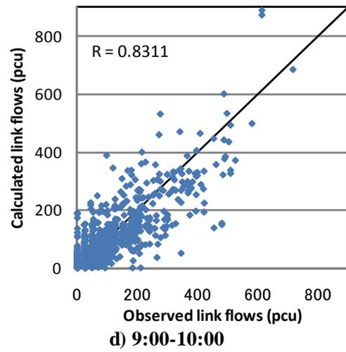
**Figure 9: Scatter plots between the observed and calculated link flows in each period**
