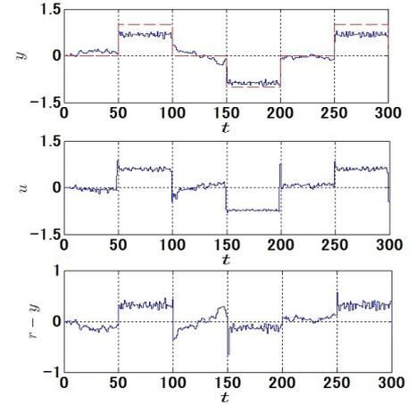
Fig. 5 Simulation result of model-free predictive control for the nonlinear system (41)
