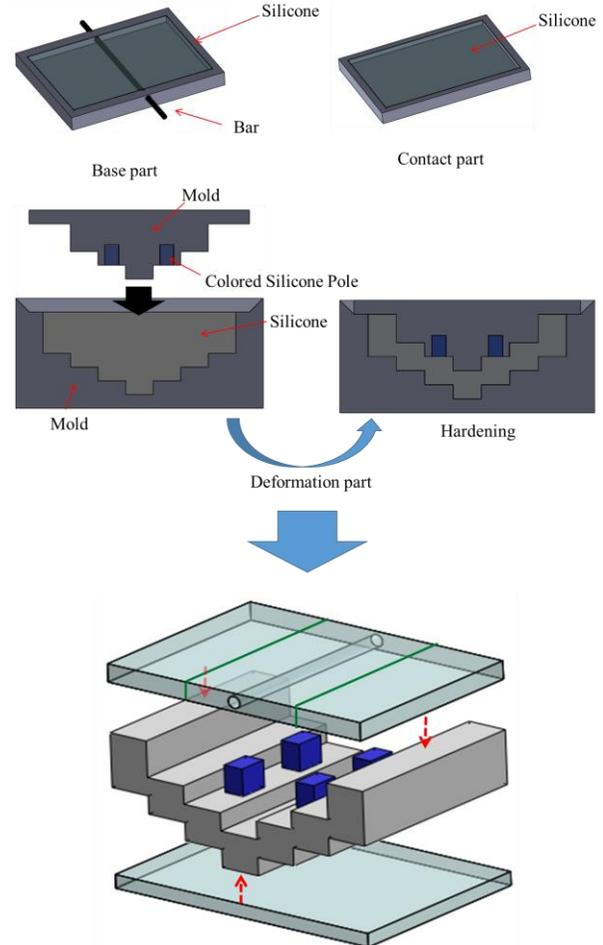
Figure 6. Overview of manufacture and assembly processes for silicone retractor with embedded force-sensing function
