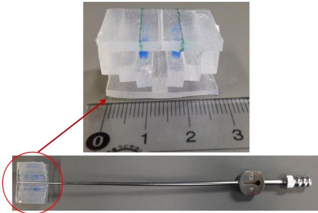
Figure 7. Manufactured silicone retractor with embedded force-sensing function
