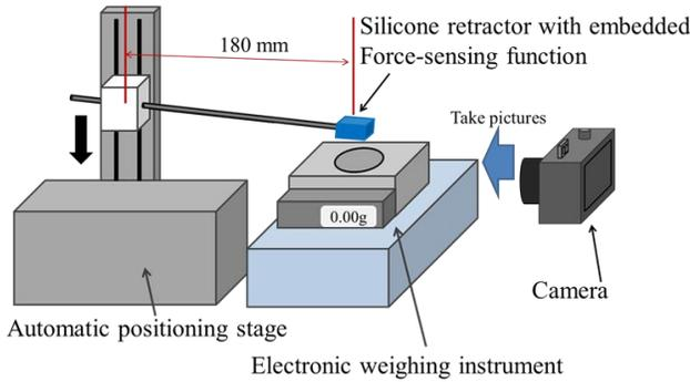
Figure 9. Schematic view of experimental setup
