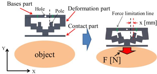
Figure 4. Principle of force sensing
