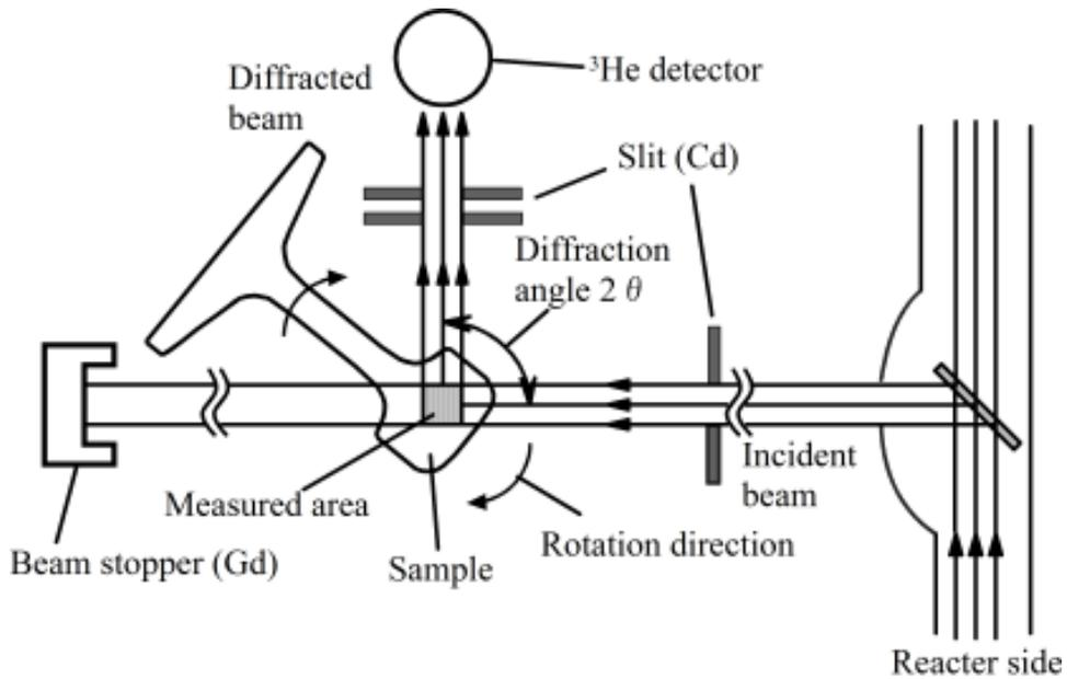
Fig. 3, Neutron optics used in this study.
