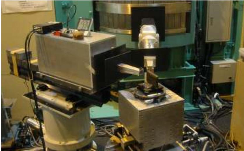
Fig. 2, Example of experimental set-up for neutron stress measurement of lattice spacing in transverse direction with RESA.
