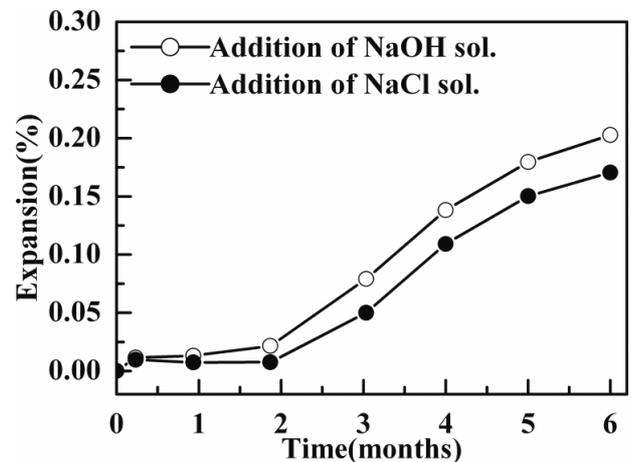
Figure 14. Expansion behaviors of concretes using recycled coarse aggregate and river sand with addition of NaOH solution and NaCl solution.
