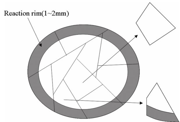
Figure 13. Schematic diagram of fragments of crushed aggregate with reaction rim.
