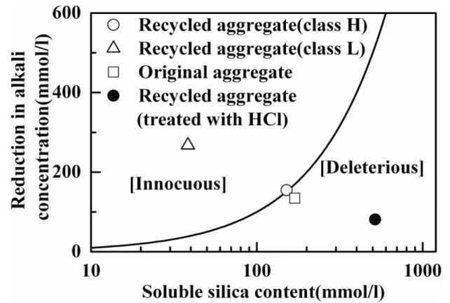
Figure 9. Results of chemical method of recycled aggregate and original aggregate (JIS A1145).
