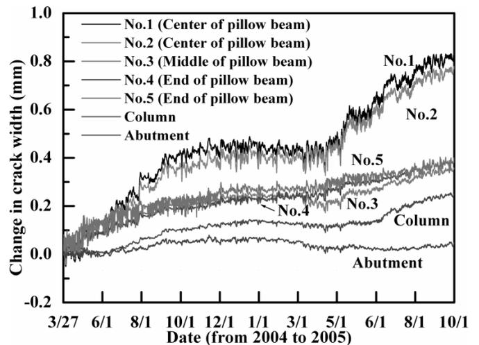
Figure 7. Variations in crack width of RC pier and abutment.
