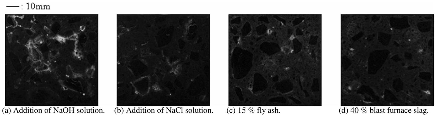
Figure 16. ASR gel observed in cross section of concrete in fog box curing.
