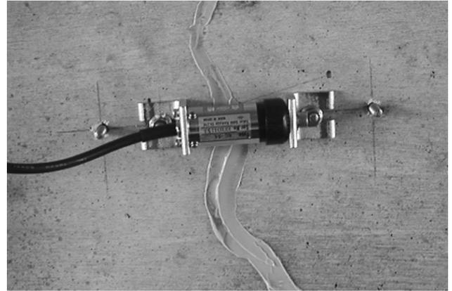
Figure 6. Sensor attached across cracks on surface of pillow beam.
