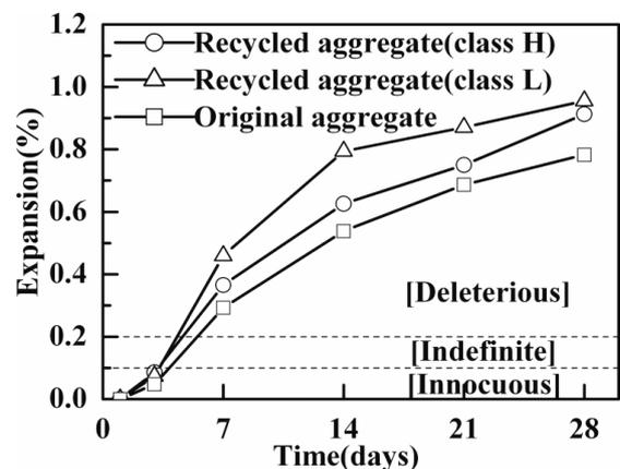
Figure 11. Expansion behaviors of mortars using recycled aggregate and original aggregate (ASTM C1260).
