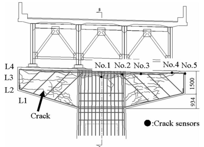
Figure 4. Schematic diagram of cracking of pillow beam.
