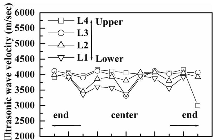
Figure 5. Change in ultrasonic wave velocity of pillow beam.
