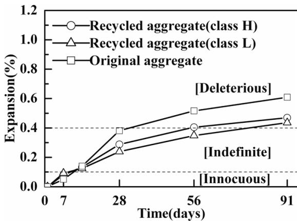
Figure 12. Expansion behaviors of mortars using recycled aggregate and original aggregate (Danish method).
