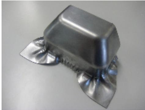
Fig.8 Wrinkling predicted in the experimental test performed with a constant BHF of 20 [kN]
