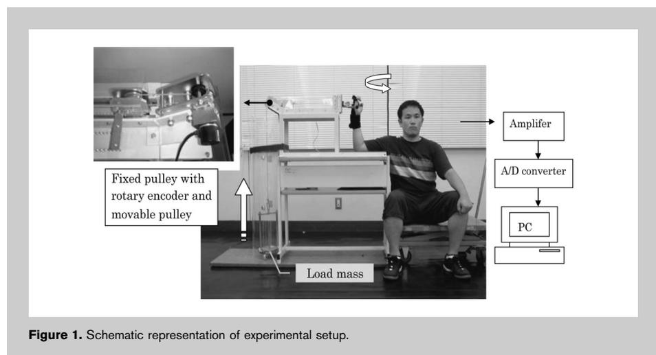
Figure 1. Schematic representation of experimental setup.
