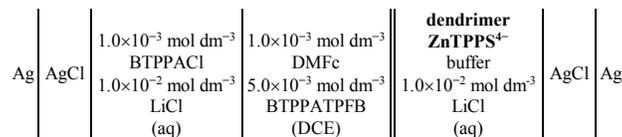
**Figure 1.** Composition of the electrochemical cell.
