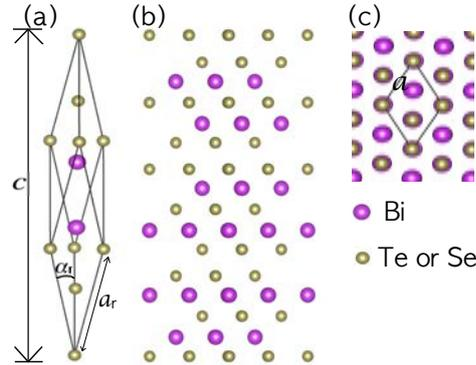
Figure 1. Crystal structure of (a) rhombohedral unit cell, (b) side view and (c) top view of hexagonal unit cell. The lattice parameters are denoted by  $a_r$  and  $\alpha_r$  for the rhombohedral unit cell and by  $a$  and  $c$  for the hexagonal one.
