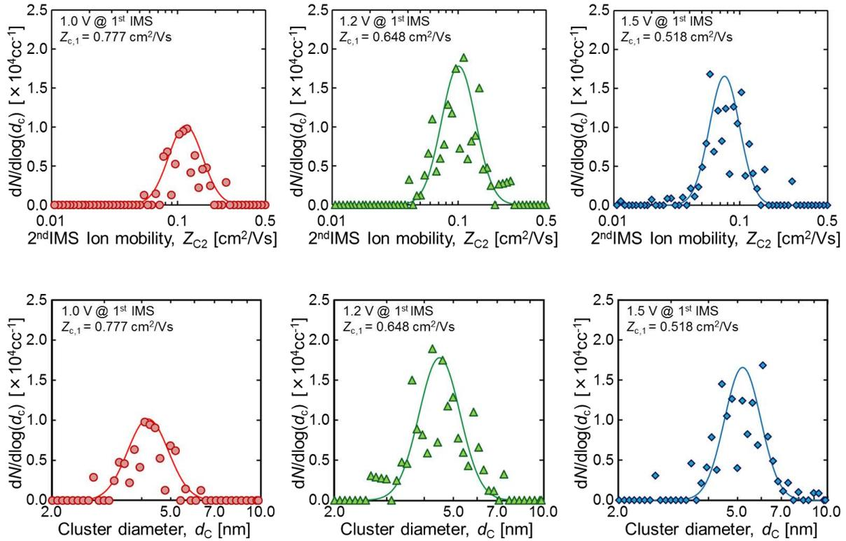
**Figure 4.** The inferred size distribution functions (in terms of the number concentration per unit log cluster diameter, obtained directly from the TSI SMPS software), as a function of inferred mobility (upper) and inferred cluster diameter (lower) from the second DMA. Results are shown for selected voltage settings in the first DMA. Symbols correspond to measured signal, with fit Gaussian curves also provided for guidance.
