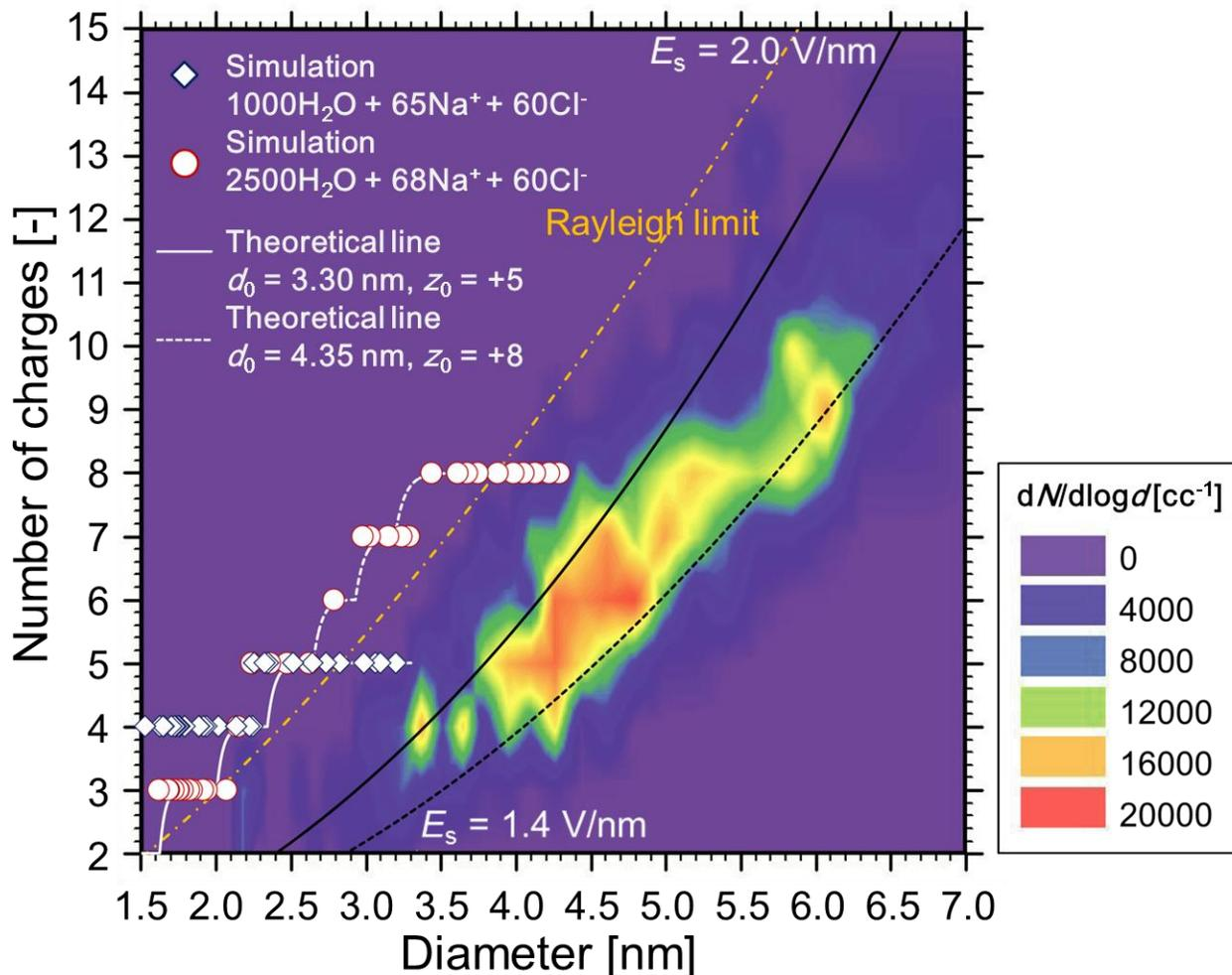
**Figure 7.** A plot of the charge state as a function of diameter from the analytical model (white lines), MD simulations (symbols), measurements (contour plot denoting size distribution function intensity), and expected for constant electric field strength models as well as at the Rayleigh limit for water.
