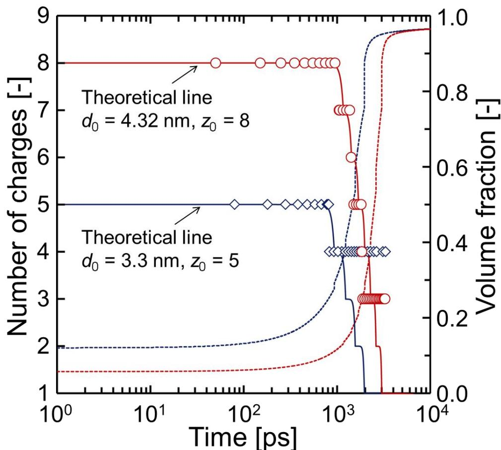
**Figure 6.** A plot of the charge state as function of simulation time for the two examined nanodrops.  $d_0$  and  $z_0$  denote the initial drop diameter and charge state. Symbols denote MD simulation results, while solid lines denote analytical model predictions. Dashed lines denote the effective sodium chloride volume fraction in drops as a function of time (right vertical axis).
