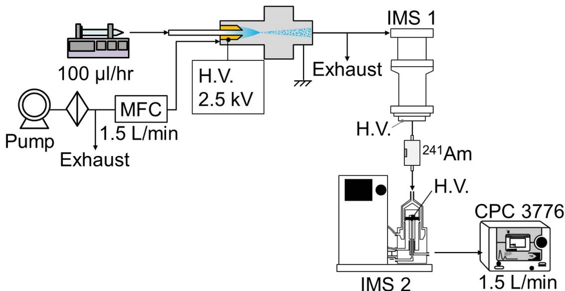
**Figure 1.** A schematic of the IMS-IMS system employed in measuring the size and charge distributions of ESI generated NaCl clusters. MFC- Mass flow controller; H.V.- High Voltage; IMS-1: A Vienna-type DMA, IMS-2: A TSI Nano-DMA (model 3085). CPC 3776: A condensation particle counter).
