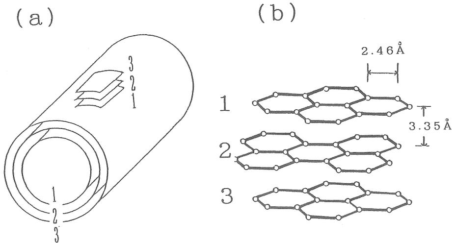
Fig. 1. (a) Schematic diagram of the structural model of the carbon nanotube reported by Iijima (1991). The number corresponds to the rolling of graphite layers.
