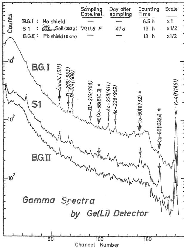
Fig. 8 The two typical background spectra with (BG II) and without (BG I) lead shield and the gamma-ray spectrum of the sea bottom soil (S-1) in Urazoko bay with lead shield
