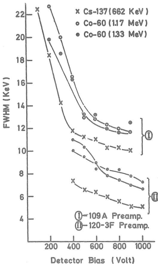
Fig. 4 The change of energy resolution (FWHM) with applied bias voltage by two different preamplifier
