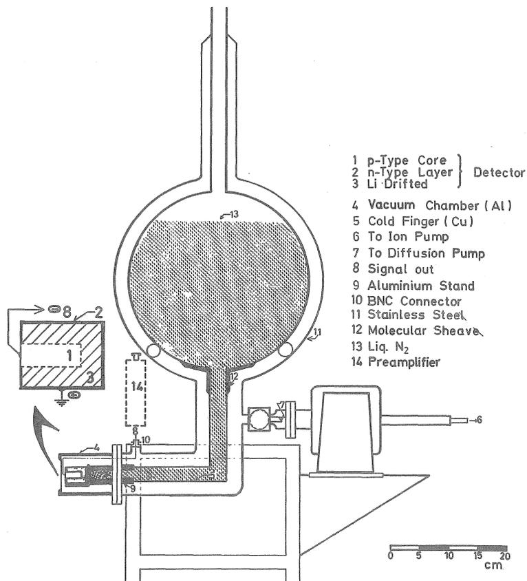
Fig. 1 Schematic illustration of the Ge (Li) detector and its cryostat
