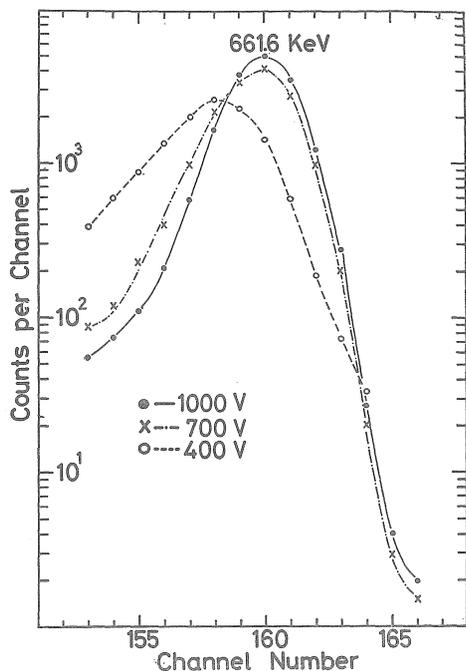
Fig. 3 The tailing effect of the Cs-137 peak as a function of applied bias voltage
