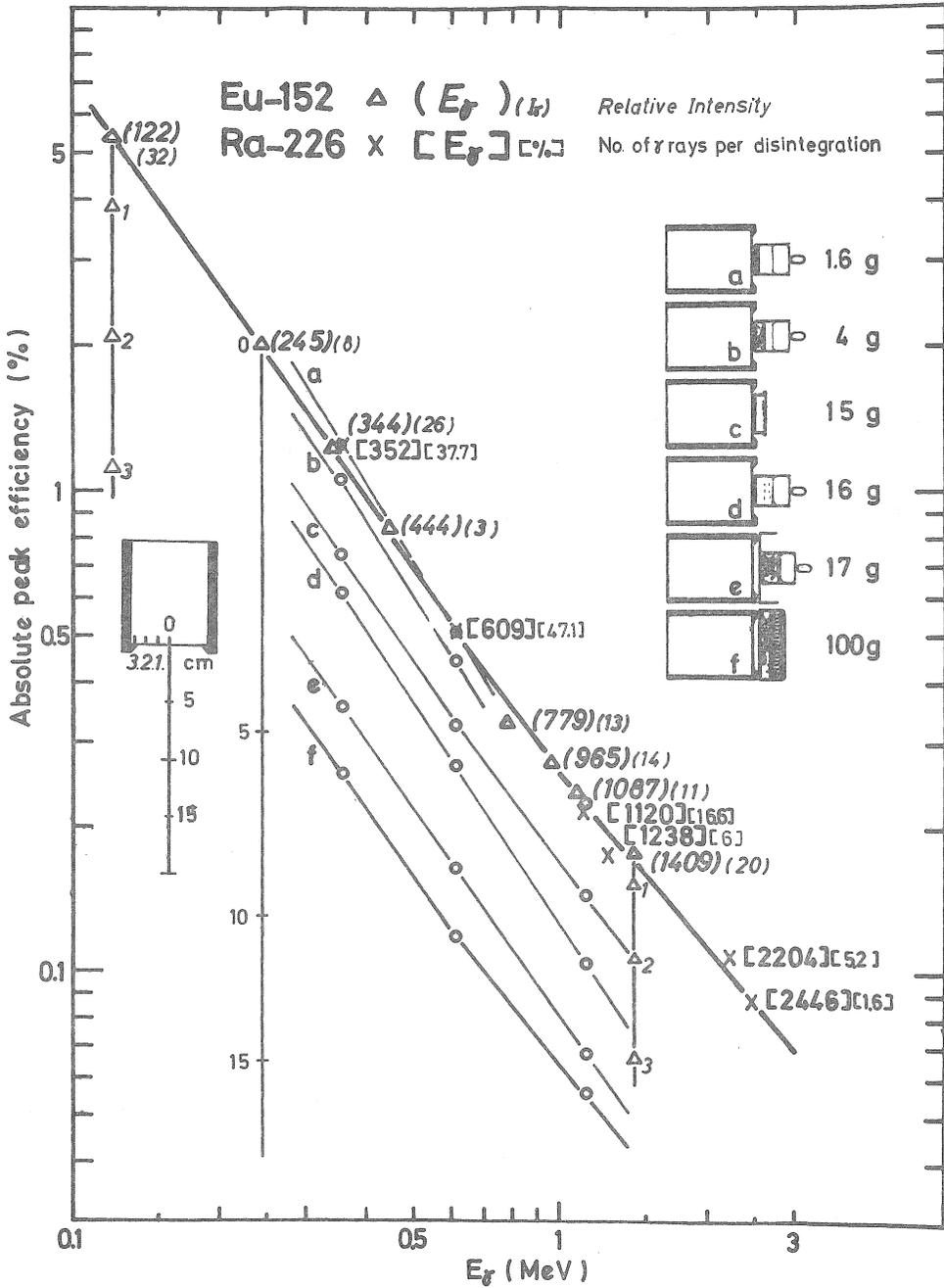
Fig. 6 The absolute peak efficiency versus both gamma-ray energy and the distance from the center of the detector head surface
