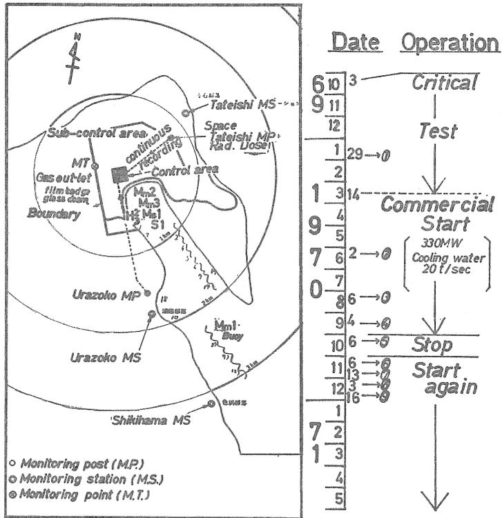
Fig. 9 The monitoring stations, several sampling locations and the records of operation of the atomic power plant at Urazoko, Tsuruga
