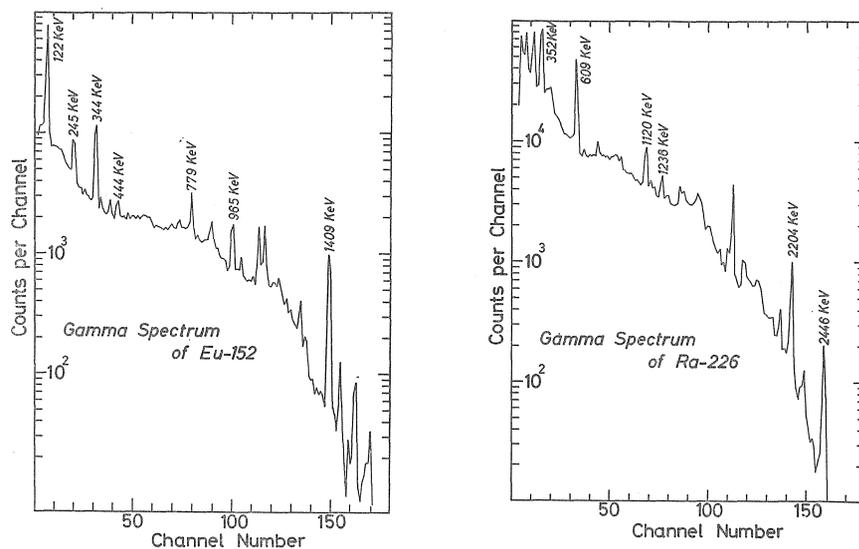
Fig. 5 The gamma-ray spectra of the gamma-ray sources, Eu-152(a) and Ra-226 with its daughter nuclides in radioactive equilibrium (b), used for relative efficiency calibration
