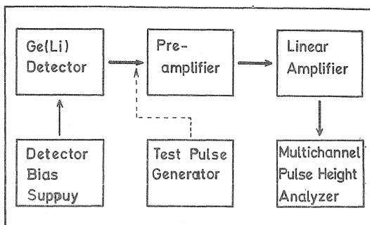
Fig. 2 Block diagram of the electronic components
