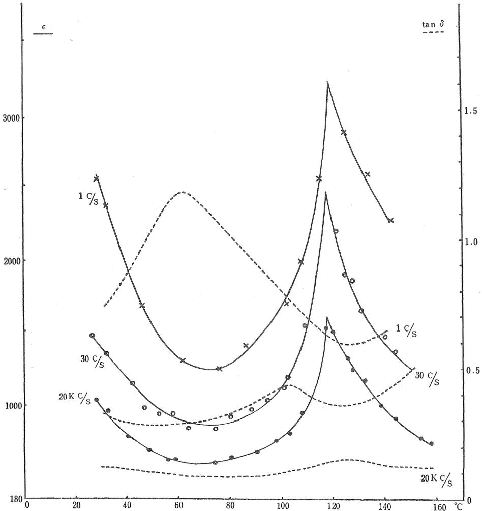
Fig. 2. Temperature dependency of dielectric constant and  $\tan \delta$
