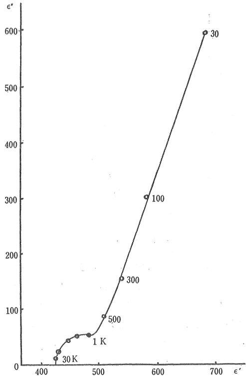
Fig. 5. Complex dielectric constant of a single crystal at 95°C.
