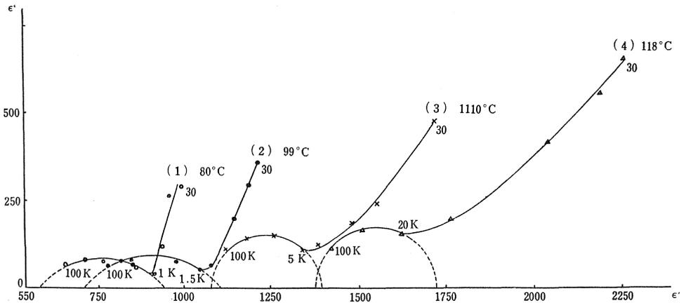
Fig. 3. Complex dielectric constant at several temperatures below Curie point
