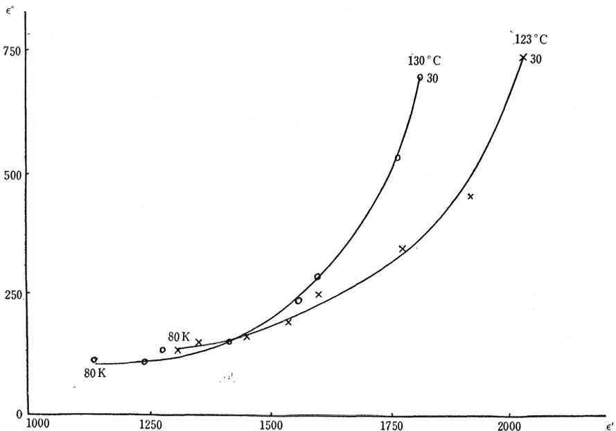
Fig. 4. Complex dielectric constant at higher temperatures than Curie point
