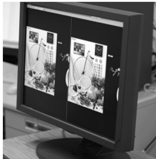
Fig.4. The newly developed resolution-enhanced 9MP LCD (TOTOKU ME351i base)
