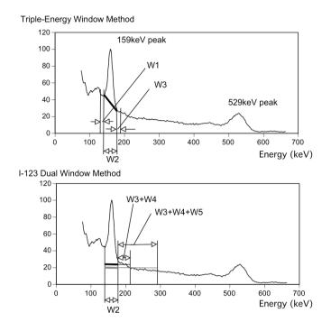
**Figure 2**Schematic representation of TEW and IDW methods. Five energy windows (W1 to W5) are shown with the energy spectrum of <sup>123</sup>I obtained with LEHR collimator. The thick lines in the W2 window indicate subtracted counts.
