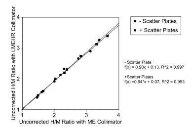
**Figure 4**Correlation between uncorrected H/M ratios with the ME and LMEHR collimators.
