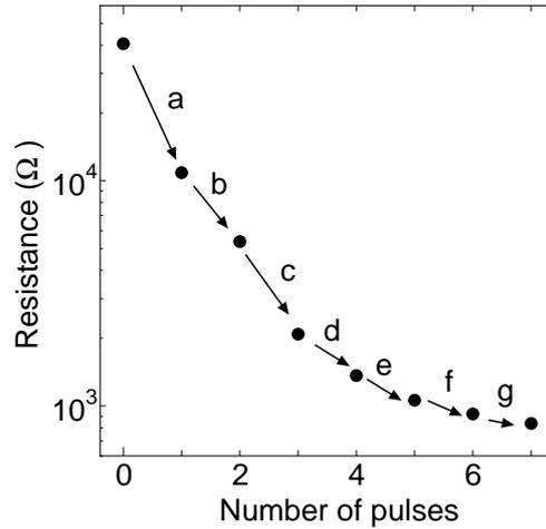
**Figure 4.** The pulse number dependency of the sample resistance. The resistance varies from 41kΩ to 840Ω with increasing the number of pulses from 0 to 7.
