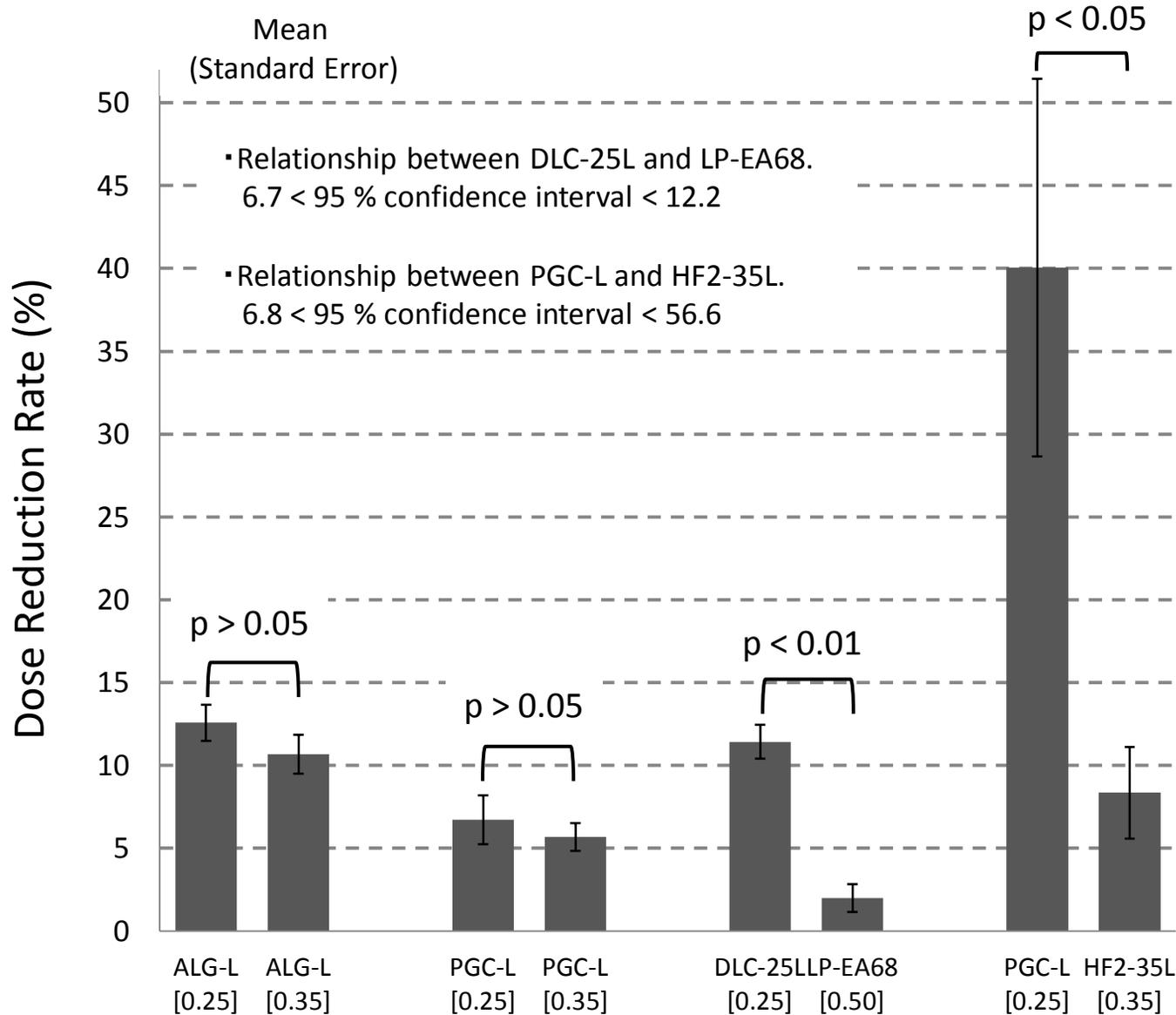
**Fig. 6** Difference in the dose reduction rate before and after the exchange of protective apron types in a practical field. ‘[ ]’ in a figure expresses the lead-equivalent thicknesses of the X-ray protective aprons.
