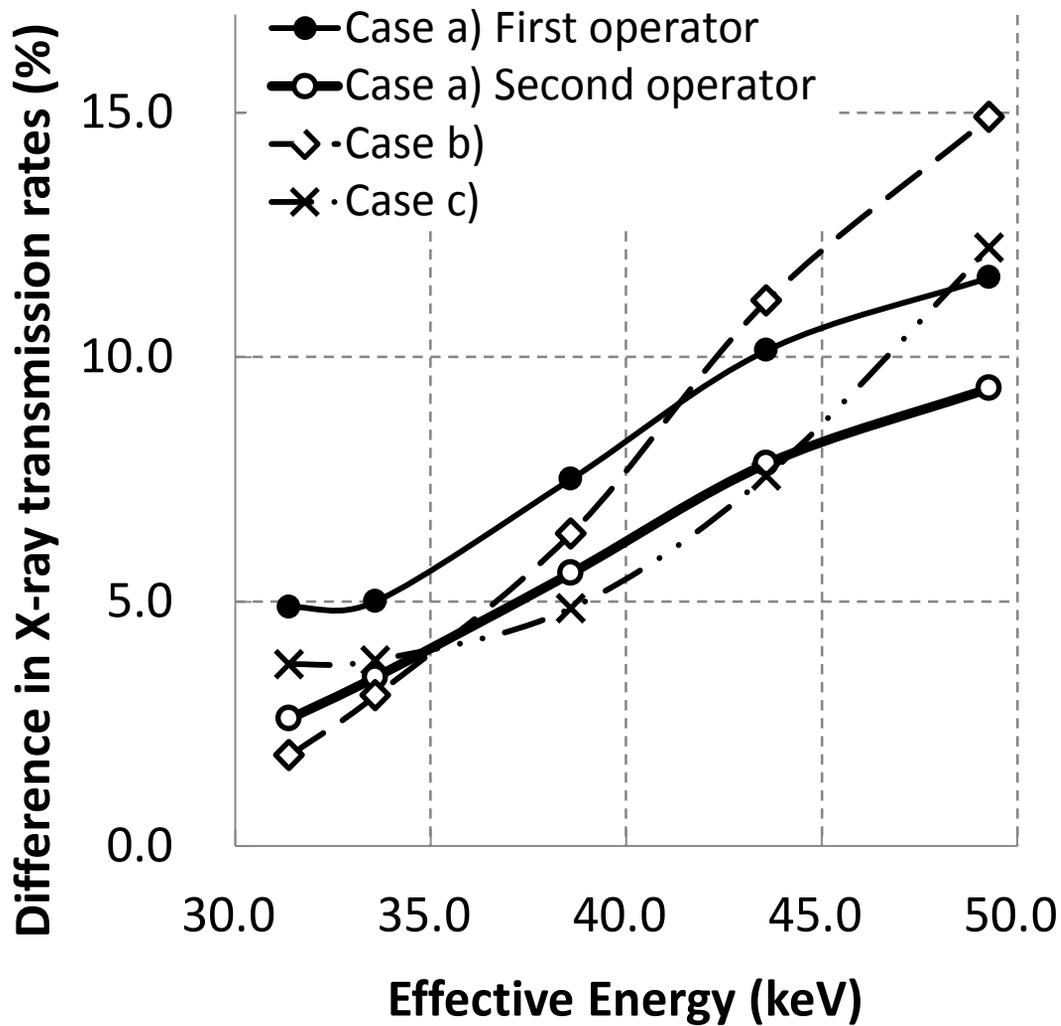
**Fig. 4** Difference in X-ray transmission rates before and after apron exchange in an experimental field. Cases a), b), and c) upon exchange of the protective apron type are described at the beginning of section 2.
