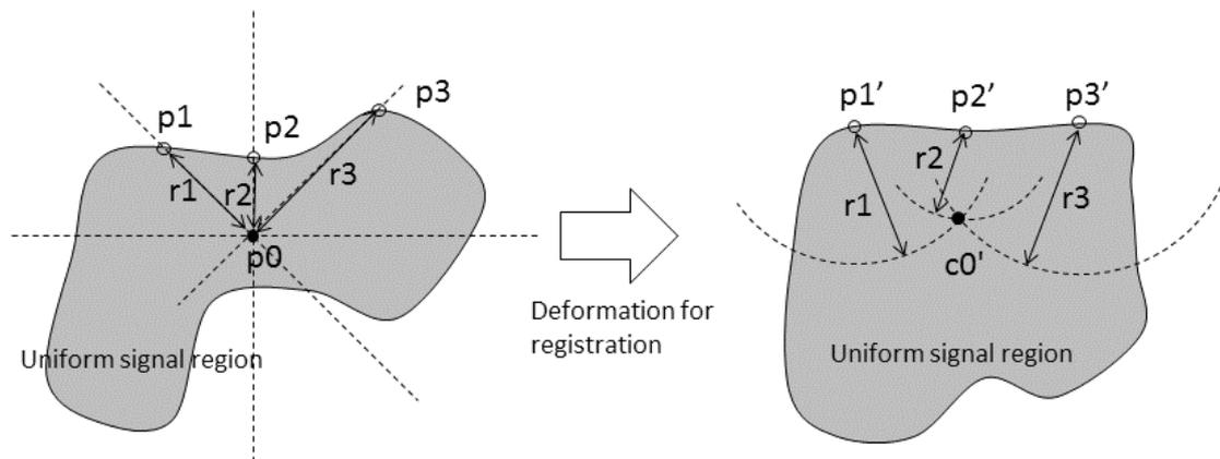
Figure 1 Schematic explanation of the candidate calculation for LU in a two-dimensional image. The  $p_0$  is a focused voxel, the  $p_1$  to  $p_3$  are surrounding voxels before DIR. After DIR, the  $p_1$  moves to  $p_1'$ , the  $p_2$  to  $p_2'$ , and the  $p_3$  to  $p_3'$ . An intersection of three circles, whose centers are  $p_1'$ ,  $p_2'$ , and  $p_3'$  and radii are  $r_1$ ,  $r_2$ , and  $r_3$ , is a candidate for the focused voxel  $c_0'$ .
