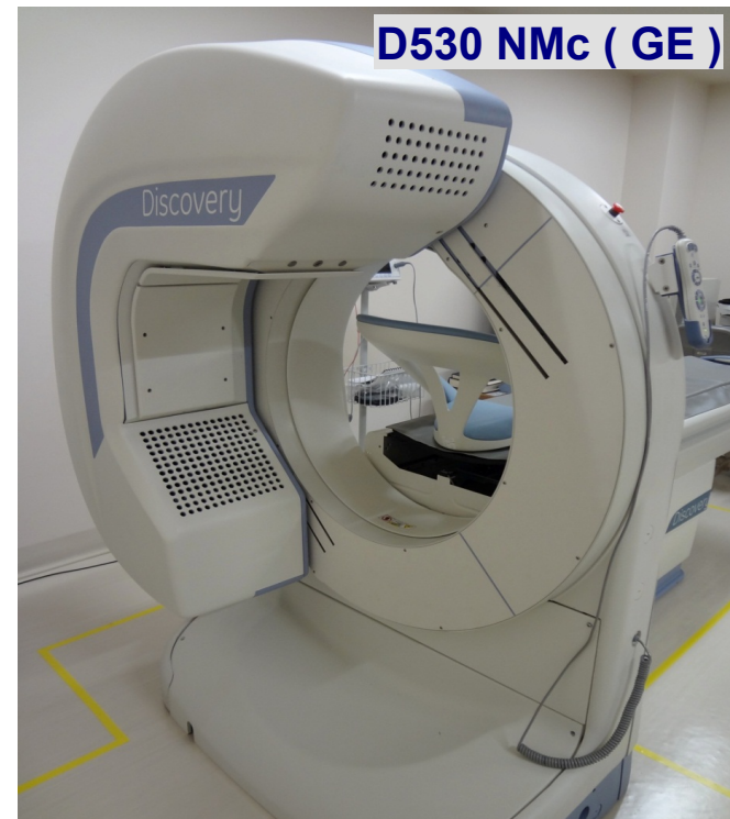
Ultrafast cardiac gamma camera with stationary semiconductor detectors
