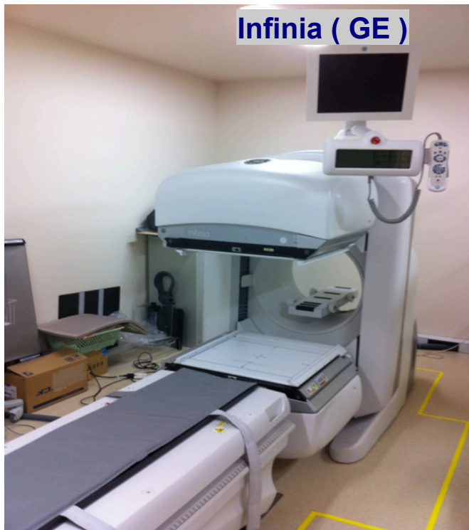
Standard Anger-type gamma camera with dual-head detectors
