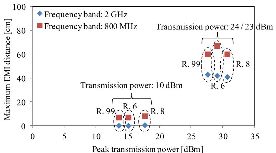
**Fig. 1.** Relationship between peak transmission power and maximum EMI distance
