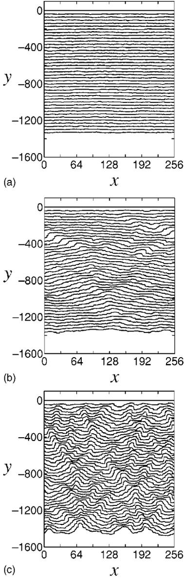
FIG. 2. Time evolution of the position of a perfectly permeable step in sublimation: (a) with the step-up drift ( $v = -0.1$ ), (b) without the drift ( $v = 0$ ), and (c) with the step-down drift ( $v = 0.1$ ).
