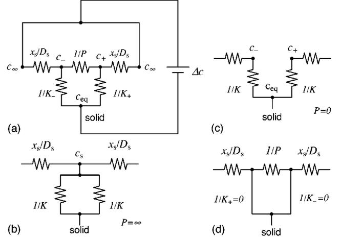
FIG. 1. Electric circuits equivalent to a single step in the super-saturated adatom density  $c_\infty$ . The resistance is defined by  $R = \Delta c / j$ , where  $j$  is the atomic current. (a) With general boundary condition. (b) For a perfectly permeable step. (c) For an impermeable step. (d) In the limit of fast step kinetics.
