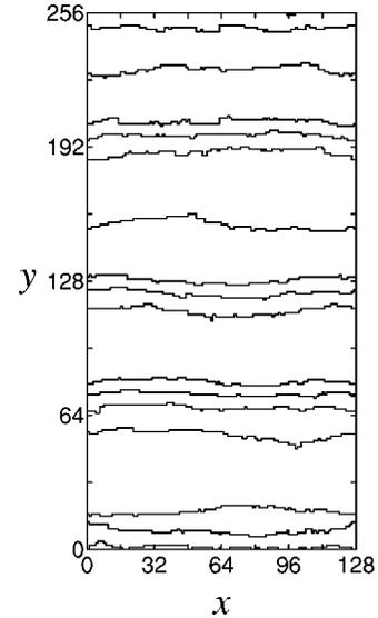
FIG. 9. A snapshot of the weak bunching of the impermeable step in sublimation at  $t = 3.7 \times 10^4$ . The step distance is longer than the surface diffusion length,  $l = 16$  and  $x_s = 8$ . The other parameters are  $A/k_B T = 10$ ,  $c_{\text{eq}} = 0.18$ , and  $\tilde{\beta}/k_B T = 2.76$ .
