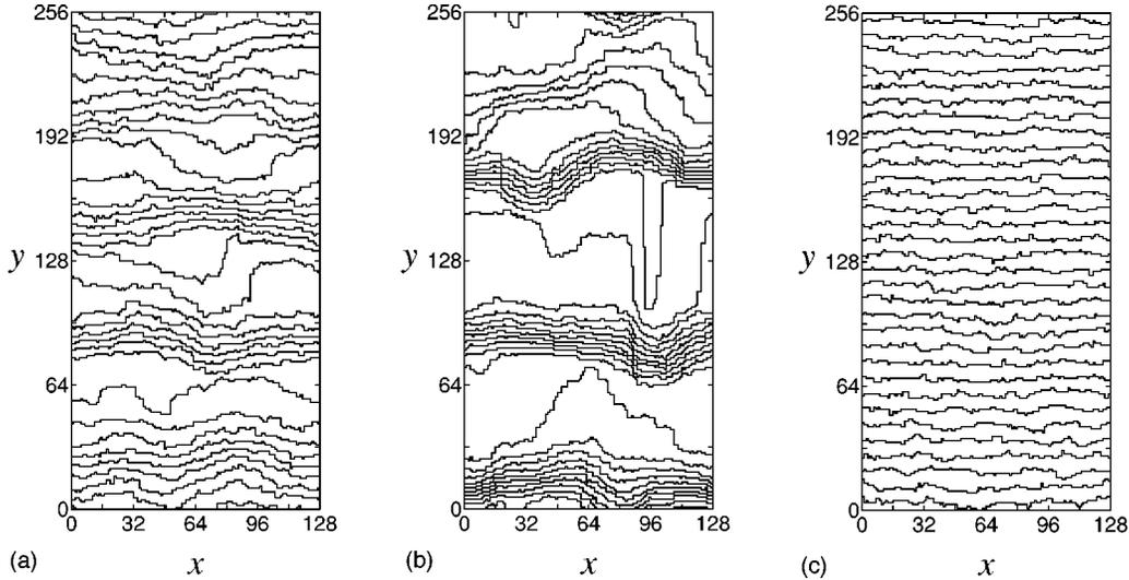
FIG. 13. Snapshots of impermeable steps in growth. The initial step distance is  $l=8$ , with  $x_s=16$ . Bunching (a) in the initial stage ( $t=1.9\times 10^4$ ) and (b) in the late stage ( $t=3.1\times 10^4$ ) with the step-down drift ( $v=0.2$ ), and (c) a stable train with the step-up drift ( $v=-0.2$ ) at  $t=3.1\times 10^4$ .
