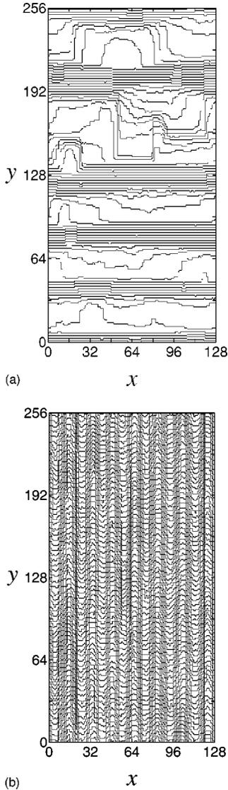
FIG. 8. Snapshots of impermeable steps in sublimation: (a) Bunching of straight steps with  $A/k_B T = 8$ ,  $l = 4$ ,  $x_s = 8$ ,  $c_{\text{eq}} = 0.18$ ,  $\tilde{\beta}/k_B T = 2.76$ , and  $v = 0.4$  at  $t = 9.5 \times 10^3$ . (b) Wandering of an equidistant step train with  $A/k_B T = 64$ ,  $l = 4$ ,  $x_s = 8$ ,  $c_{\text{eq}} = 0.18$ ,  $\tilde{\beta}/k_B T = 0.13$ , and  $v = 0.4$  at  $t = 1.8 \times 10^4$ .
