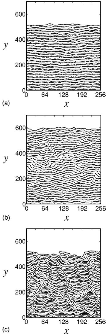
FIG. 10. Time evolution of the position of a permeable step in growth. The impingement rate is  $F = 2 \times 10^{-3}$ , (a) with the step-up drift ( $v = -0.2$ ), (b) without the drift, and (c) with the step-down drift ( $v = 0.2$ ).
