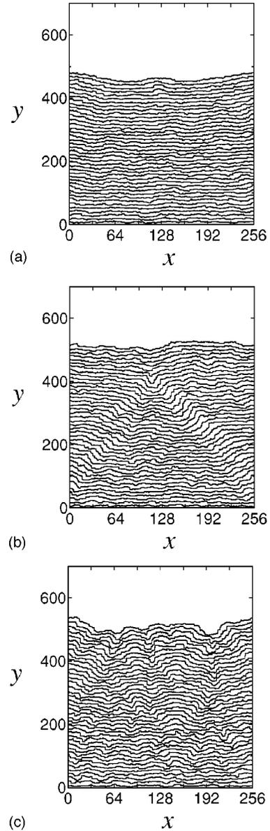
FIG. 11. Time evolution of the position of an impermeable step in growth. The impingement rate is  $F = 2 \times 10^{-3}$ , (a) with the step-down drift ( $v = 0.2$ ), (b) without drift, and (c) with the step-up drift ( $v = -0.2$ ).
