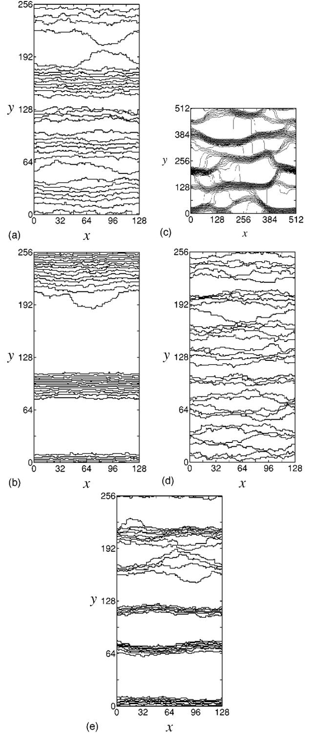
FIG. 6. Snapshots of bunching of permeable steps in sublimation: (a) in the initial stage ( $t = 5.6 \times 10^4$ ), (b) in the late stage ( $t = 8.2 \times 10^4$ ), and (c) in the late stage ( $t = 1.0 \times 10^5$ ) in a large system, with the step-up drift ( $v = -0.6$ ) and repulsive interaction ( $A/k_B T = 4.0$ ). (d) In the initial stage ( $t = 4.1 \times 10^3$ ), and (e) in the late stage ( $t = 2.1 \times 10^4$ ), with the step-up drift ( $v = -0.6$ ) and no repulsive interaction.
