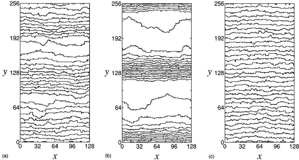
FIG. 12. Snapshots of bunching of permeable steps with the repulsive interaction  $A/k_B T = 10$  in growth, (a) in the initial stage ( $t = 9.6 \times 10^4$ ) and (b) in the late stage ( $t = 1.9 \times 10^5$ ) with the step-down drift ( $v = 0.4$ ), and (c) at  $t = 3.8 \times 10^4$  with the step-up drift ( $v = -0.4$ ),
