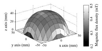
Fig. 8. Reconstructed magnetic field distribution.
