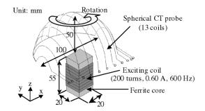
Fig. 6. Experimental target and CT probe.
