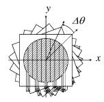
Fig. 3. Multilayered magnetic CT probe [5].
