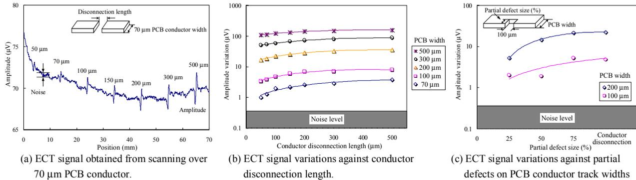
Fig. 3 ECT signal variation on different kinds of defect.
