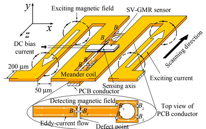
Fig. 2 Proposed SV-GMR based ECT probe.
