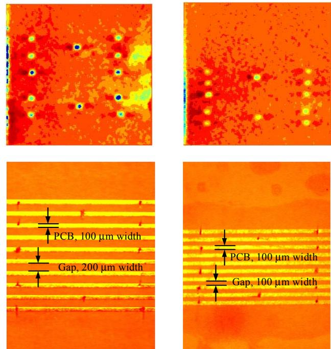
Fig. 4 PCB model (lower) and scanning result (upper).
