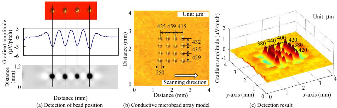
Fig. 7 Identification of the conductive microbead (PbSn) position, conductive microbead array model and its detection results.
