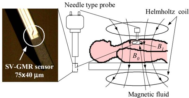
Fig. 8 Application of needle type SV-GMR to estimate volume density of magnetic fluid.
