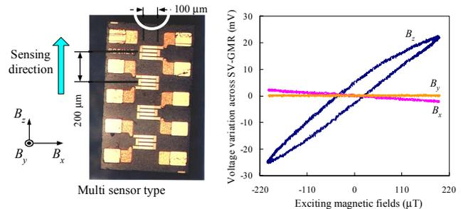
Fig. 1 Proposed SV-GMR and characteristics.
