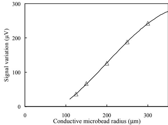
Fig. 6 Signal variation vs. microbead (PbSn) radius.
