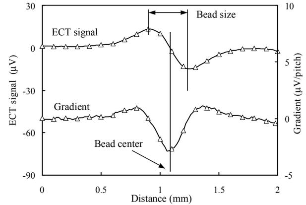
Fig.5 ECT signal obtained from the detection of a conductive microbead (PbSn) with 125  $\mu\text{m}$  radius and its signal gradient.
