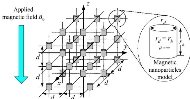
Fig. 9 Model of magnetic nanoparticles uniformly distributed inside magnetic liquid.
