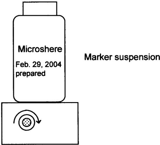
Never shaking and accelerating the magnetic stirrer, not to bubble up!
