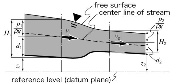
$H$  is flow depth. The mean flow velocity is substitutable for the flow velocity at the center line.
