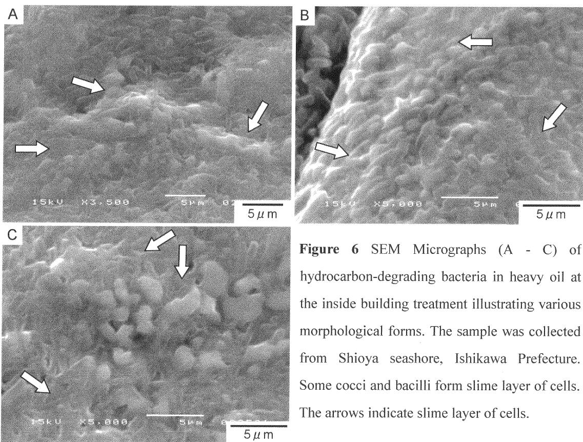
**Figure 6** SEM Micrographs (A - C) of hydrocarbon-degrading bacteria in heavy oil at the inside building treatment illustrating various morphological forms. The sample was collected from Shioya seashore, Ishikawa Prefecture. Some cocci and bacilli form slime layer of cells. The arrows indicate slime layer of cells.
