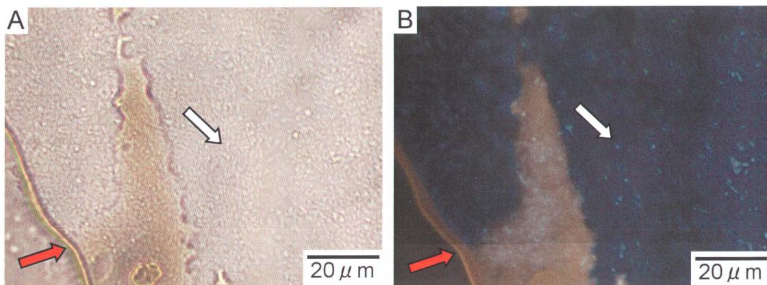
**Figure 1** Optical micrographs of hydrocarbon-degrading bacteria in association with oil droplets at the inside building treatment. The sample was collected from Shioya seashore, Ishikawa Prefecture. The white arrow indicates bacteria, and the red arrow indicates heavy oil droplet designated by the brown color in the figure. (A) A differential interference microscopic image. (B)
