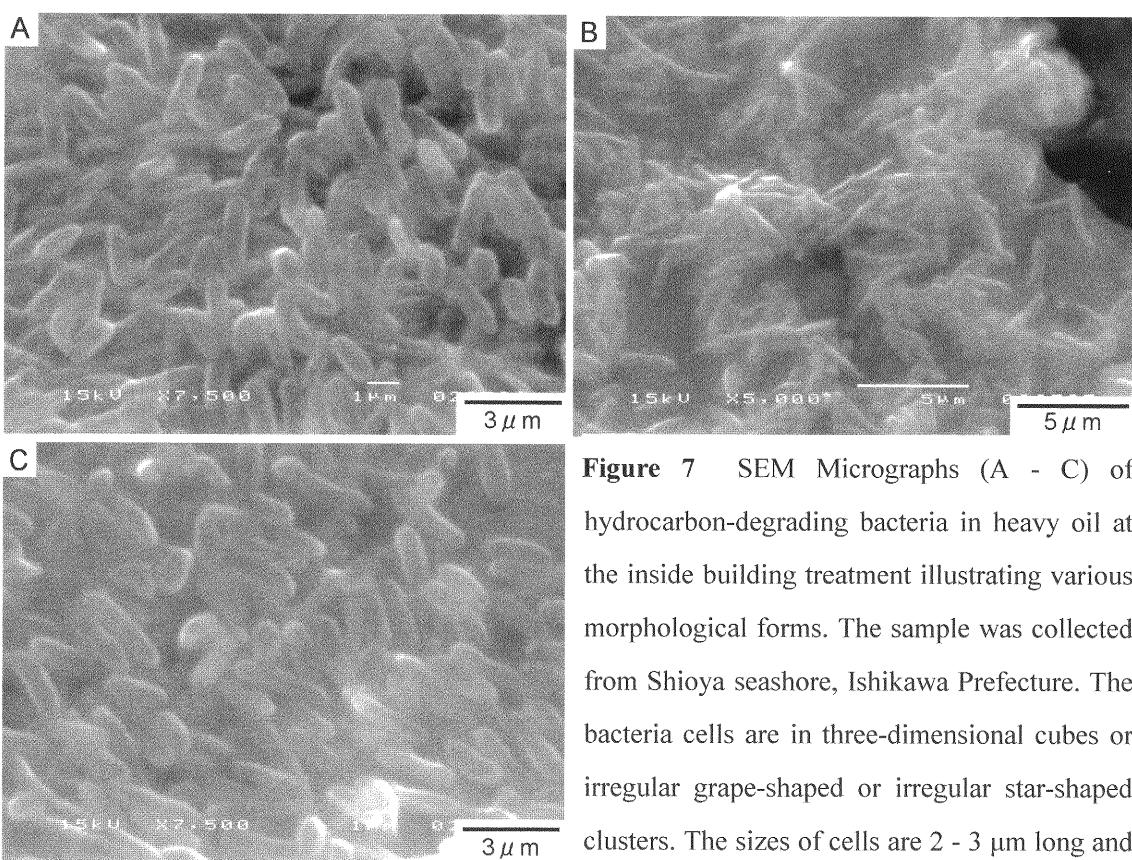
**Figure 7** SEM Micrographs (A - C) of hydrocarbon-degrading bacteria in heavy oil at the inside building treatment illustrating various morphological forms. The sample was collected from Shioya seashore, Ishikawa Prefecture. The bacteria cells are in three-dimensional cubes or irregular grape-shaped or irregular star-shaped clusters. The sizes of cells are 2 - 3 μm long and 0.5 - 1 μm wide.
