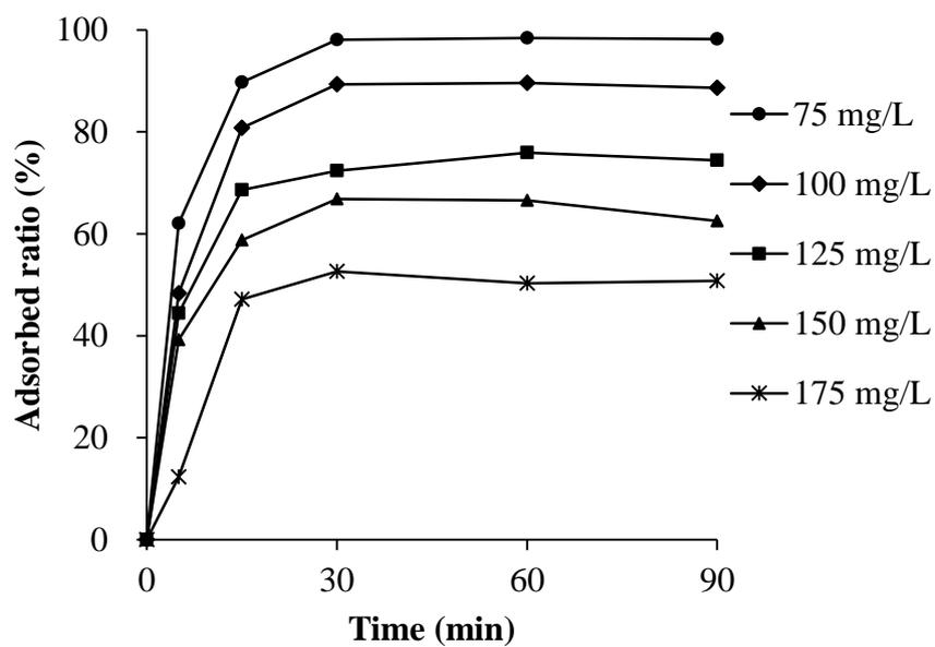
**Fig. 4.6** Effect of contact time and initial MB concentration on MB adsorption, for differing initial MB concentrations. pH: 11; FPT gel dose: 0.03 g/20 mL solution; temperature: 30 °C
