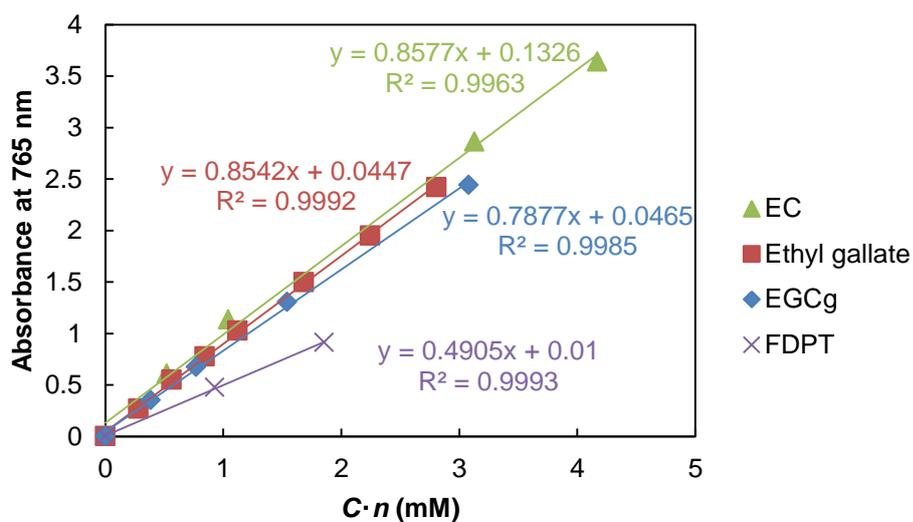
**Fig. 2.10** Comparative calibration curves for Folin-Ciocalteus's assay with EC, ethyl gallate and EGCg standards and PT sample. Subunit composition of PT was estimated based on phloroglucinol decomposition.
