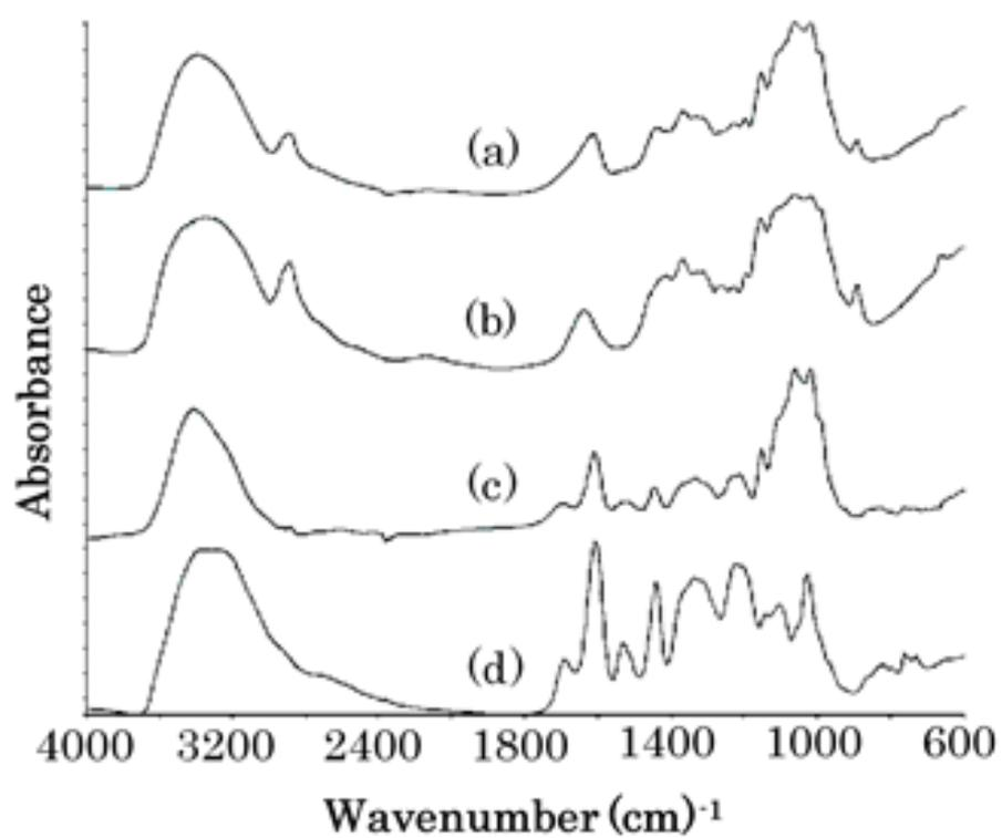
**Fig. 5.1** IR spectra of (a) day 42 PTIC gel, (b) cellulose viscopearl, (c) subtraction of (b) from (a), (d) freeze-dried PT
