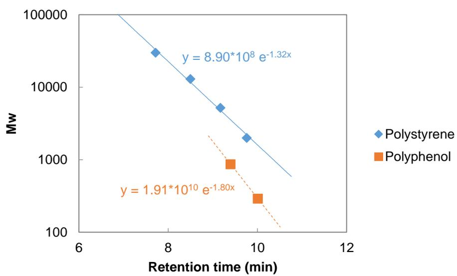
Fig. 2.7 Calibration curves based on polystyrene and polyphenols.
