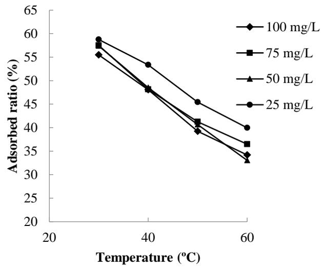
**Fig. 3.7** Effect of temperature on the adsorption of caffeine for the initial caffeine concentration of 100 mg/L, the PT gel dose of 1 g/20 mL, and contact time of 30 min
