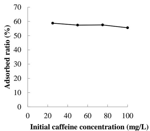
**Fig. 3.5** Effect of initial concentration on the adsorption of caffeine at 30 °C, the PT gel dose of 1 g/20 mL, contact time of 30 min
