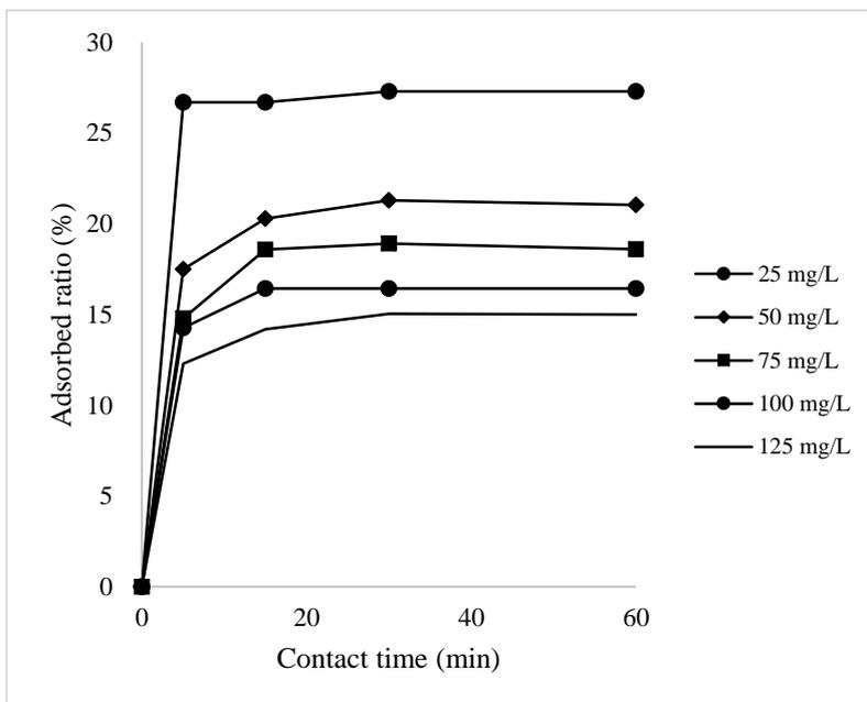
**Fig. 5.4** Effect of contact time on the adsorption for different initial concentrations of caffeine at 30°C and day 42 PTIC gel dose of 0.25g/ 20 mL
