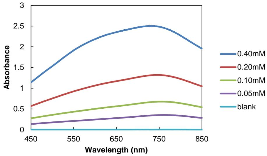
**Fig. 2.9** Visible adsorption spectra of the reaction mixtures of (-)-EGCg Folin-Ciocalteu's phenol reagent on Folin-Ciocalteu's assay
