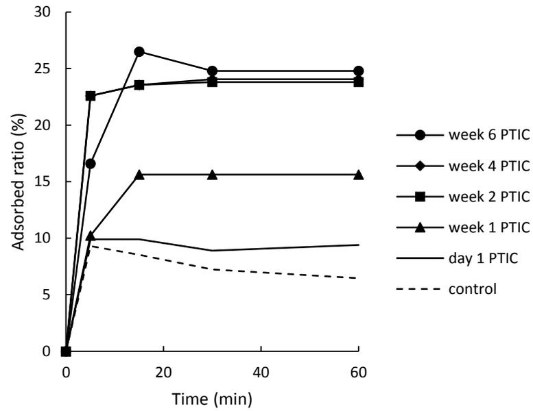
**Fig. 5.2** Adsorbed ratio of day 1, week 1, week 2, week 4, and week 6 PTIC gel and cellulose viscopearl (control) at 30 °C, 50 mg/L of caffeine solution, and 0.25 g of adsorbent dosage
