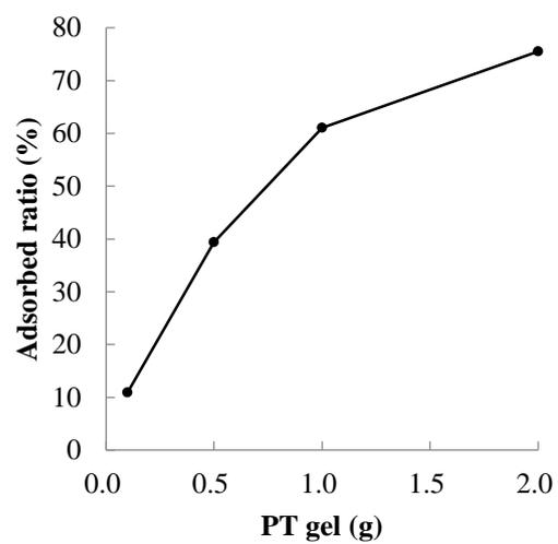
**Fig. 3.6 Effect of the PT gel dose on the adsorption of caffeine for initial caffeine concentration of 100 mg/L, contact time of 30 min, and temperature of 30 °C**
