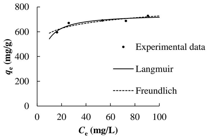
**Fig. 4.9** The fit of the experimental data of RBO adsorption on APT gel to the Langmuir and Freundlich models. pH: 3; APT gel dose: 0.03 g/20 mL solution; contact time: 60 min; temperature: 30 °C
