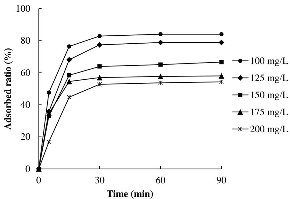
**Fig. 4.7 Effect of contact time and initial RBO concentration on RBO adsorption, for differing initial RBO concentrations. pH: 3; APT gel dose: 0.03 g/20 mL solution; temperature: 30 °C**
