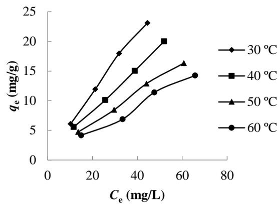
**Fig. 3.8** Adsorption isotherm of caffeine on the PT gel
