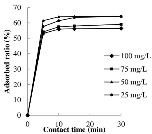
**Fig. 3.4** Effect of contact time on the adsorption of caffeine for different initial concentration at 30 °C, the PT gel dose of 1 g/20 mL
