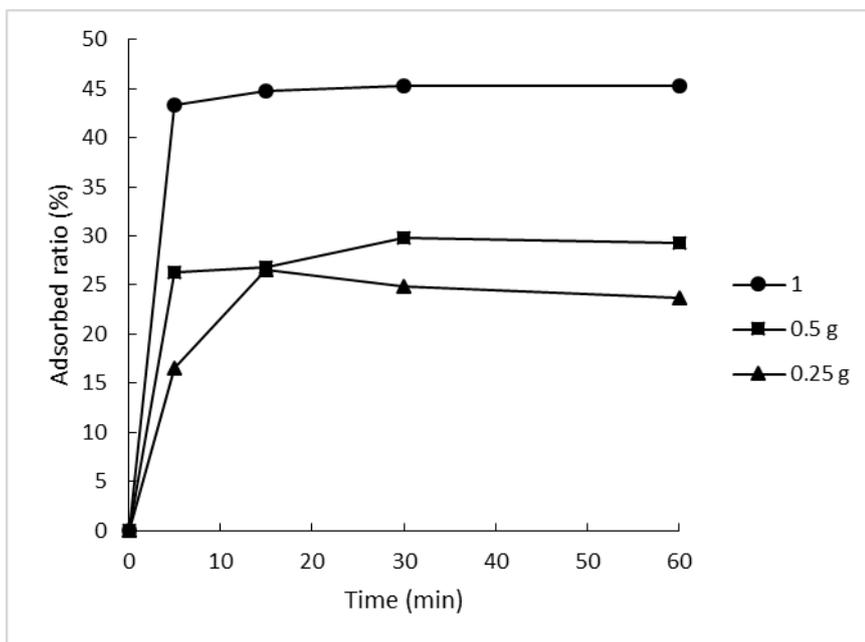
**Fig. 5.3** Effect of day 42 week PTIC gel dose on adsorption of caffeine at 30° C and initial concentration of 50 mg/L.
