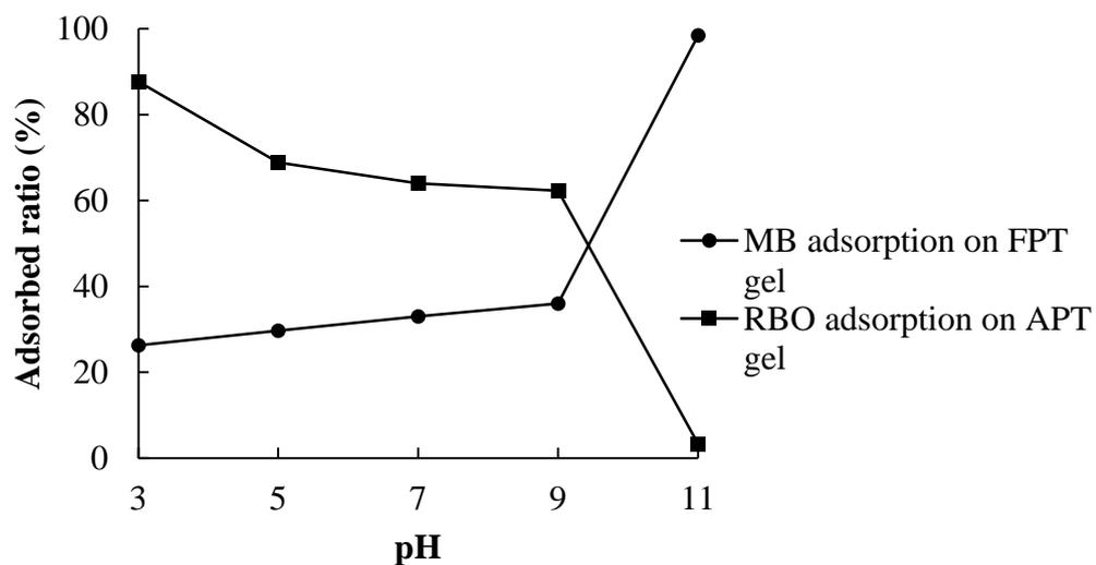
**Fig. 4.5 Effect of pH on FPT adsorption for MB and APT adsorption for RBO. Initial dyes concentration: 100 mg/L; FPT and APT gel dose: 0.05 g/20 mL and 0.03 g/20 mL solution, respectively; contact time: 60 min, temperature: 30 °C**
