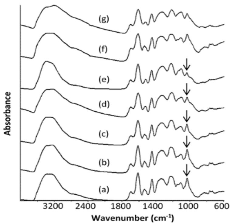
**Fig. 4.4** IR spectra of (a) freeze-dried PT, (b)-(e) FPT gels prepared from 0.02, 0.2, 2.0 and 20% concentration formaldehyde solutions, respectively, (f) APT gels prepared from 0.02% formaldehyde solution and 6.6 mg ammonium chloride, and (g) APT gels prepared from 2.0% formaldehyde solution and 0.66 g ammonium chloride
