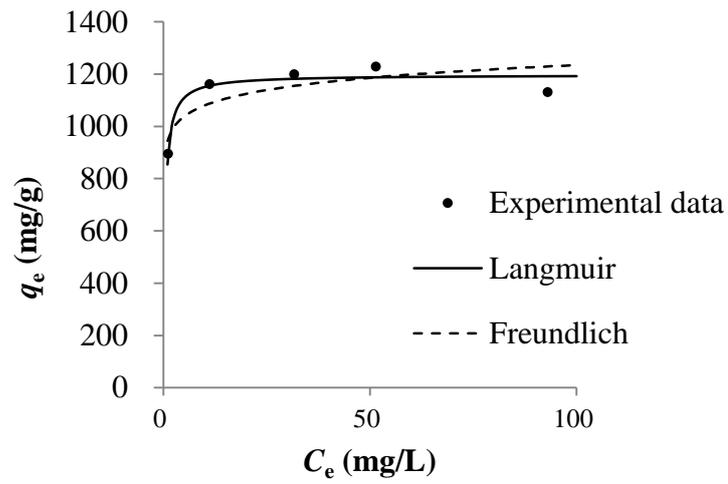
**Fig. 4.8** The fit of the experimental data of MB adsorption on FPT gel to the Langmuir and Freundlich models. pH: 11; FPT gel dose: 0.03 g/20 mL solution; contact time: 60 min; temperature: 30 °C
