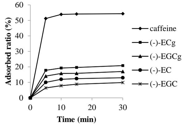
**Fig. 3.3 Adsorption of caffeine and catechins on the PT gel: initial concentration of caffeine and catechins of 100 ppm, gel dose of 1 g/20 mL, contact time of 30 minutes, temperature of 30 °C**
