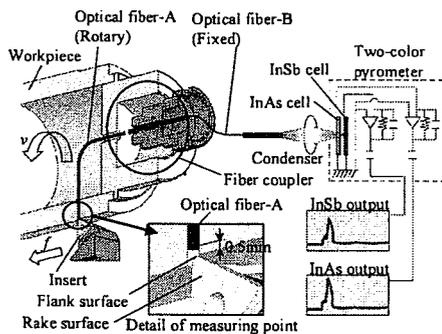
Fig.1 Structure of fiber-coupled two-color pyrometer equipped for turning
