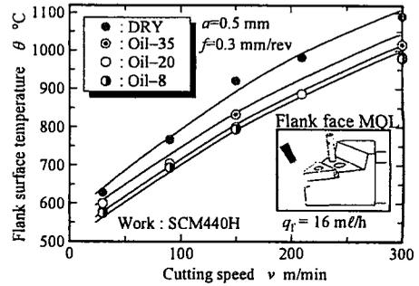
Fig.15 Effect of oil mist supplied to tool flank face on tool temperature
