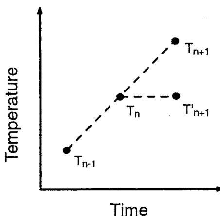
Fig. 1 Method of Estimation for Nodal Temperature
