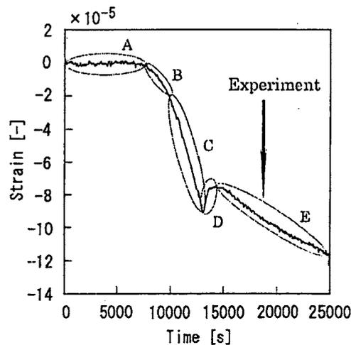
Fig. 8 Circumferential Strain in Experiment at 80 °C
