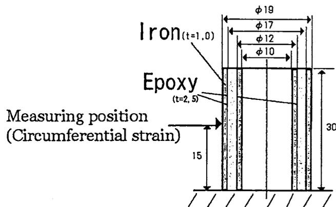
Fig. 7 Cross-sectional view of test pieces (unit:mm)
