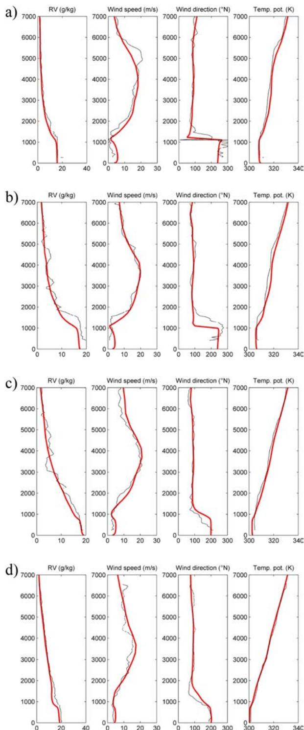
**Fig. 7.** Vapour mixing ratio (g/kg), wind speed (m/s) wind direction (deg) and potential temperature (K) derived from dropsonde measurements (red lines) and the MESONH simulation (black lines) at 12° N (a, DS1), at 10° N (b, DS2), at 8° N (c, DS3) and at 6° N (d, DS4) on 13 June.
