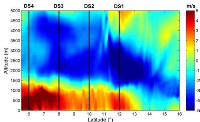
**Fig. 6.** Vertical cross section (along the ATR-42 flight track at 2.00° E) of the meridional component of the simulated wind (m/s). The black lines indicate the location of the dropsondes released by the F-F20 along the transect. The numbers refer to the dropsonde numbers as they appear in Fig. 7.
