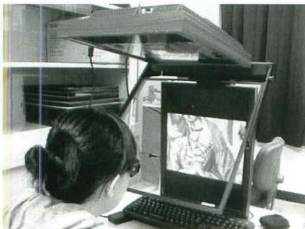
Fig. 14 Observation of stereo images using 3-Dmonitor
