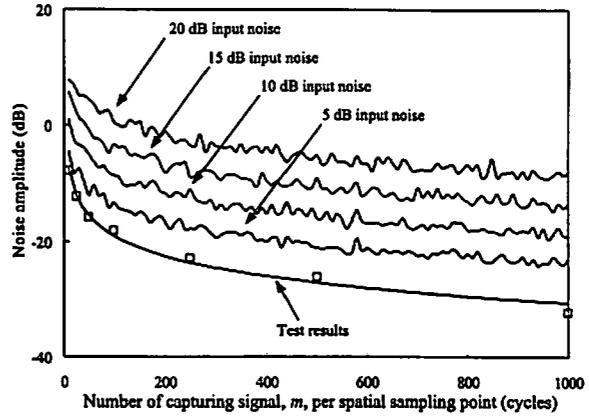
Fig. 3. Signal to noise ratio rejection performance by applied Fourier transform
