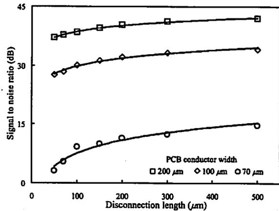
Fig. 5. Signal to noise ratio vs. conductor disconnection length acquired by Lock-in amplifier.
