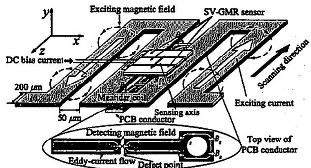
Fig. 1. Proposed ECT probe model with multi SV-GMR sensor
