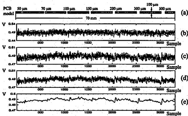
Fig. 7. Detected ECT signal with SV-GMR scanning over PCB model (a) with scanning speed of 0.05 m/s and 200-cycle capturing signal,  $m$ . (b) detected signal from SV-GMR, (c) applied 5-averaging signals, (d) applied 9-averaging signal, and (e) applied FIR filter to signal (d)
