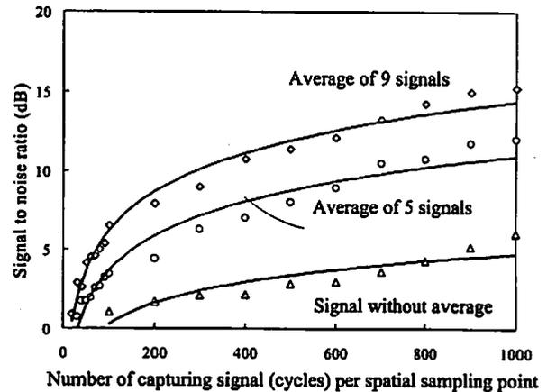
Fig. 4. Simulation results of SNR improvement with proposed technique (defect signal: -20 dB, noise: 10 dB)
