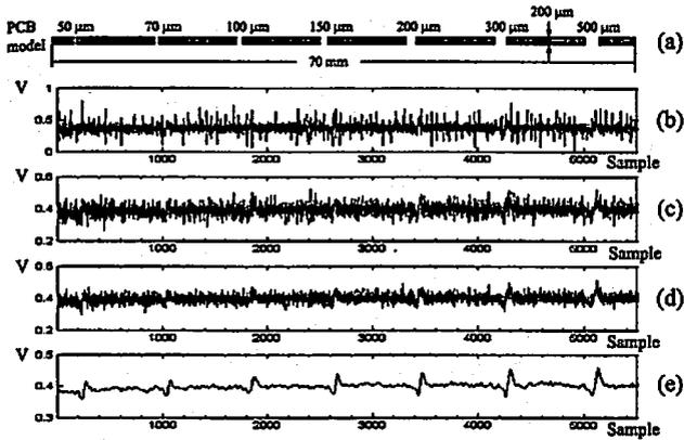
Fig. 6. Detected ECT signal with SV-GMR scanning over PCB model (a) with scanning speed of 0.10 m/s and 10-cycle capturing signal,  $m$ . (b) detected signal from SV-GMR, (c) applied 5 averaging signals, (d) applied 9-averaging signal, and (e) applied FIR filter to signal (c)
