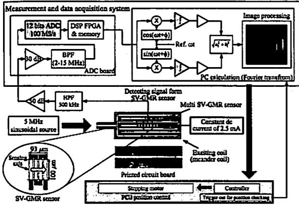
Fig. 2. Proposed system configuration
