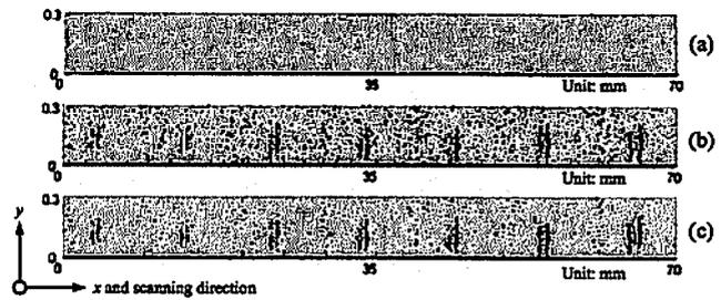
Fig. 8. Two-dimension gradient image obtained from scanning the PCB model in Fig. 6 (a) with scanning speed of 0.05 m/s and 200-cycle capturing signal,  $m$ . (a) the result without applied averaging technique, (b) 5-averaging signal result, and (c) 9-averaging signal results
